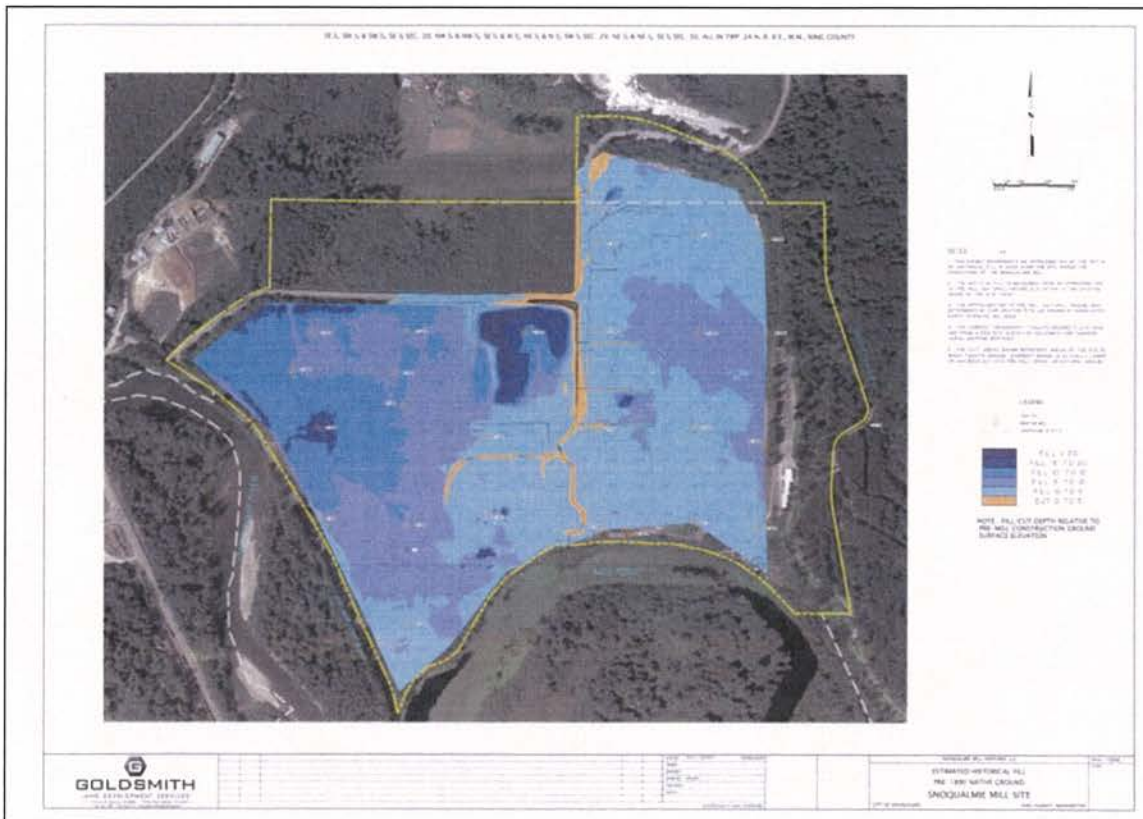
Figure 3. Estimated historical fill / Pre-1890 Native Ground of the Snoqualmie Mill Site, provided by Snoqualmie Mill Ventures, LLC.
