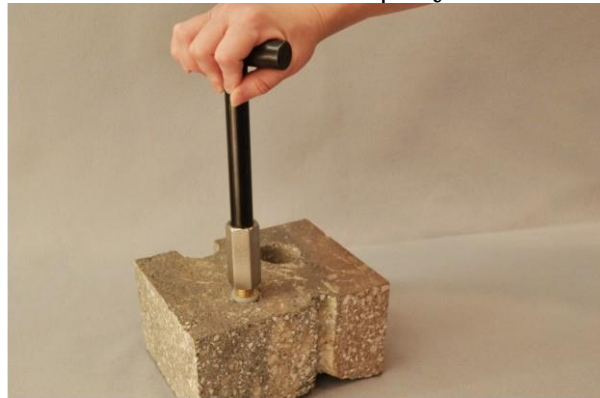
Figure 7. Removing the VAPOR PIN®
