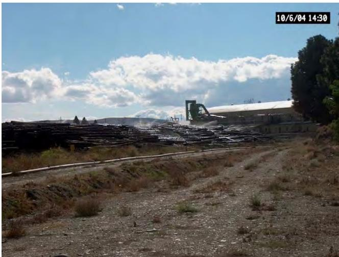
Log deck water sprinkler equipment consisted of common agricultural aluminum hand lines that were placed a top the log decks. The sprinkler lines were connected to a pressurized aluminum main line along the perimeter of the log decks, visible in the photograph as a long series of piping from the left of the photograph. This photograph was collected south of the river water intake with the former planer building in the background.
