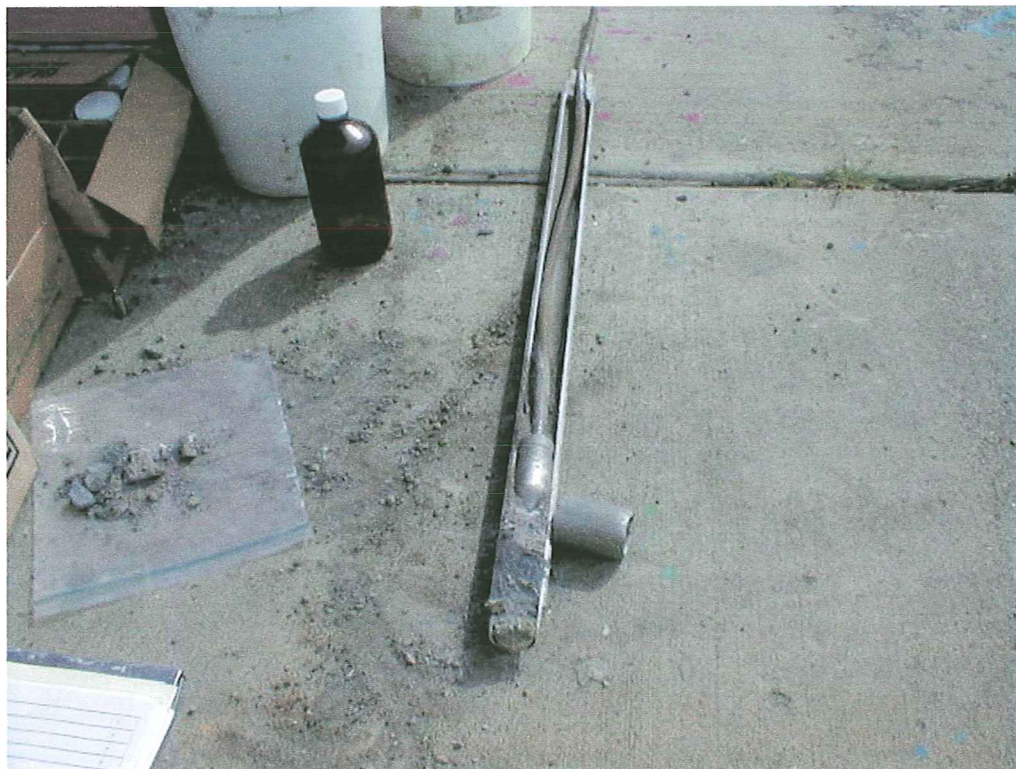
PHOTO 4: VERY DENSE SOIL FROM BORING #2
