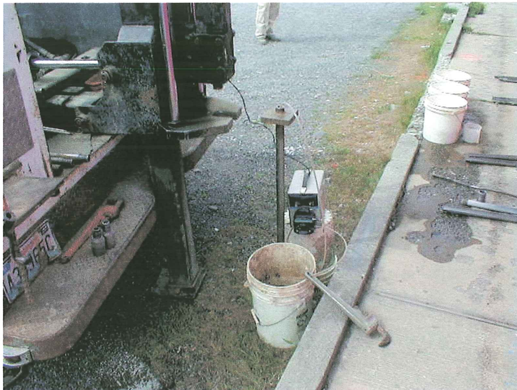
PHOTO 3: GROUNDWATER SAMPLING WITH PERISTALTIC PUMP
