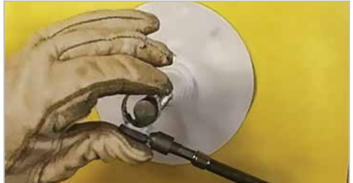
STEP 6. Hose Clamp Loosely Installed
