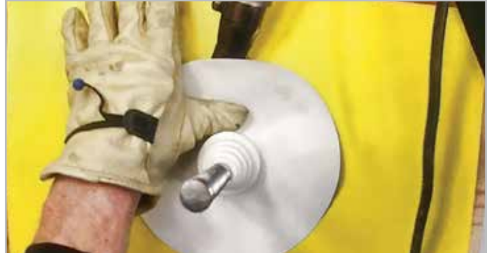
STEP 5. Tack weld PF-150 flange
