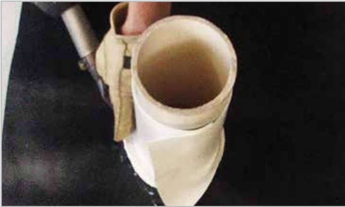
STEP 4. Final weld NR to target piece
