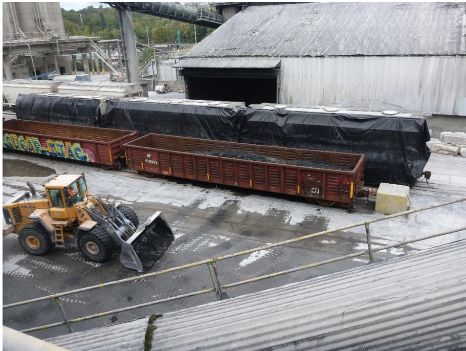
**Photograph 38: Dredge sediment railcar loading operations.
