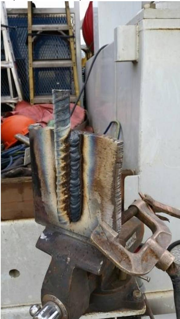
Completed Weld Test Coupon
