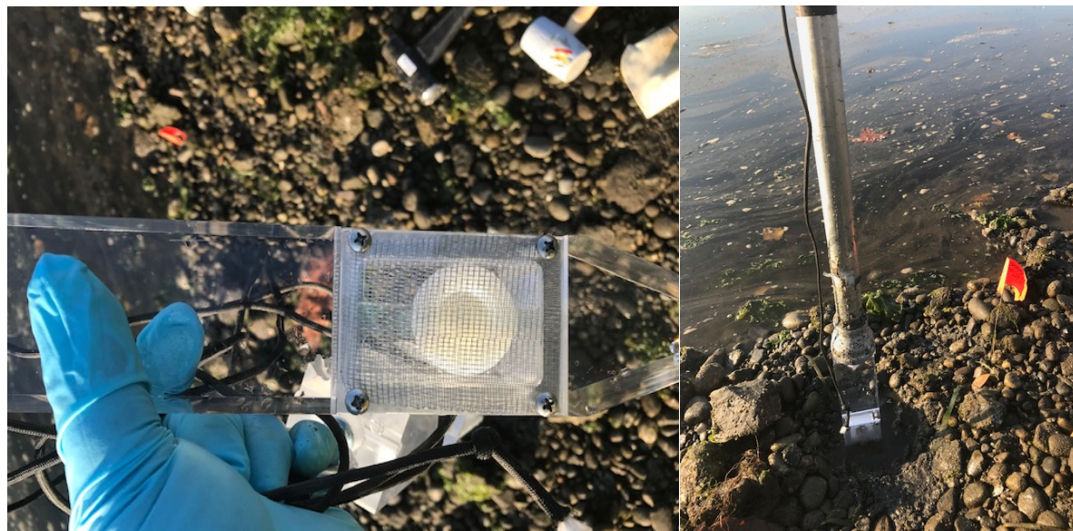
Figure 8 Probe with DGT Piston Assembly Installed (left) and Probe Installation (right)
