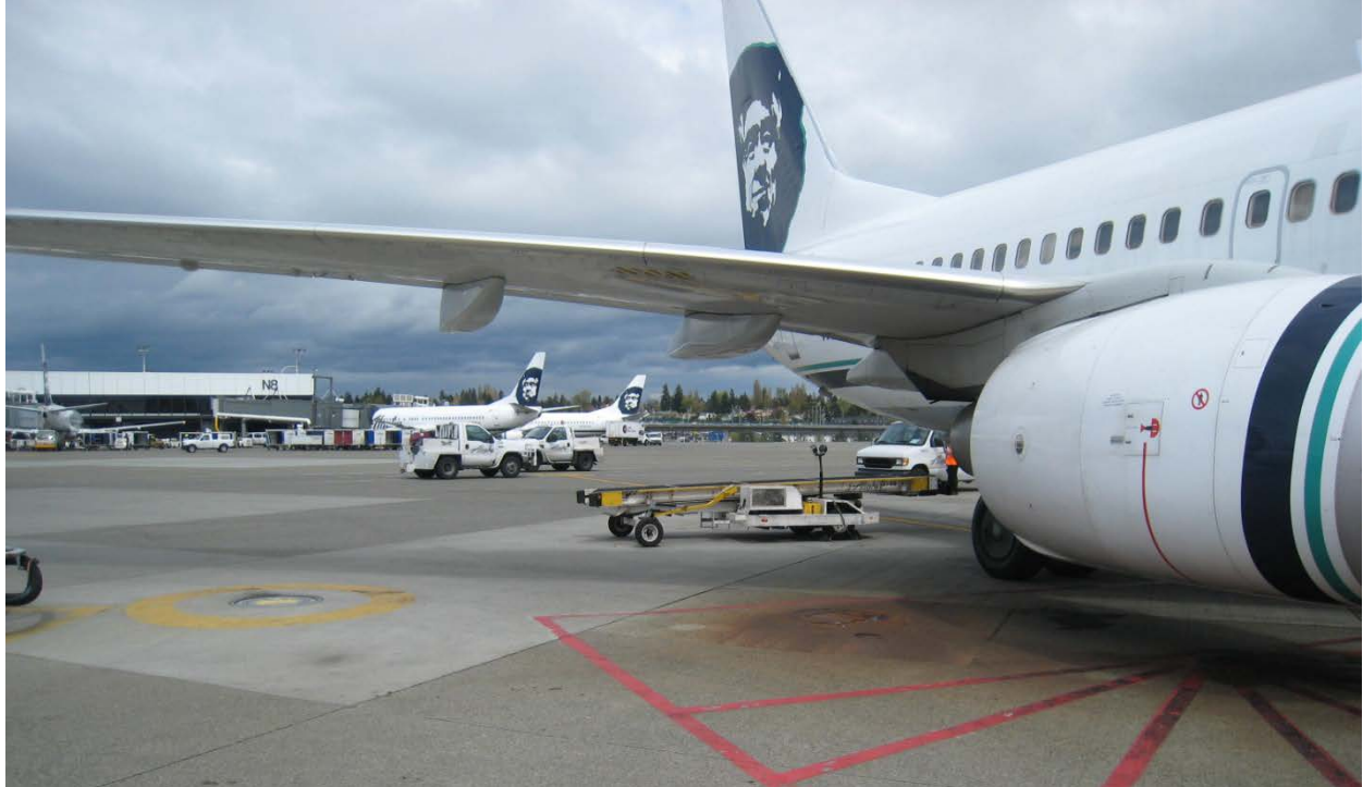
Photo 3: New hydrant fuel line access pt. at left (yellow circle). Old one is in the rusty spot.
