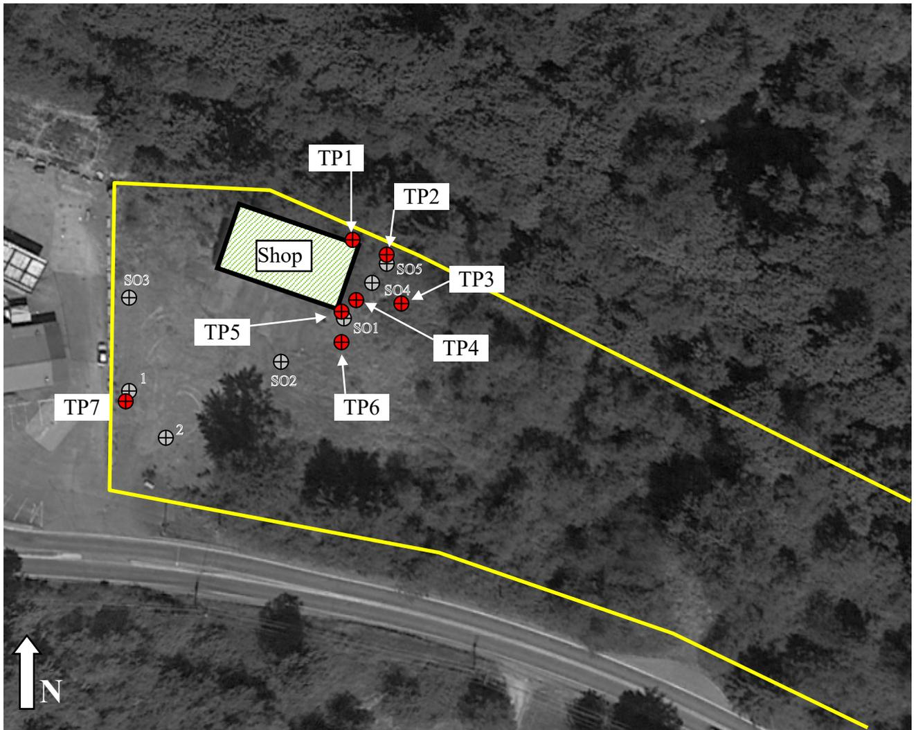
**Figure 6.** Sample results from test pit investigation, July 2008
