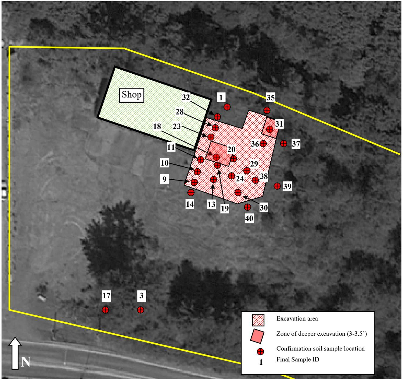
**Figure 8.** Confirmation soil sample locations from 2018 soil cleanup
