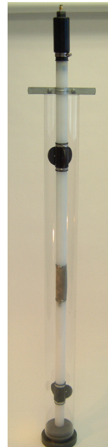
Figure 2 CMT model assembly in 4.75" (12 cm) acrylic cylinder, later filled with sand and used in grout testing.
