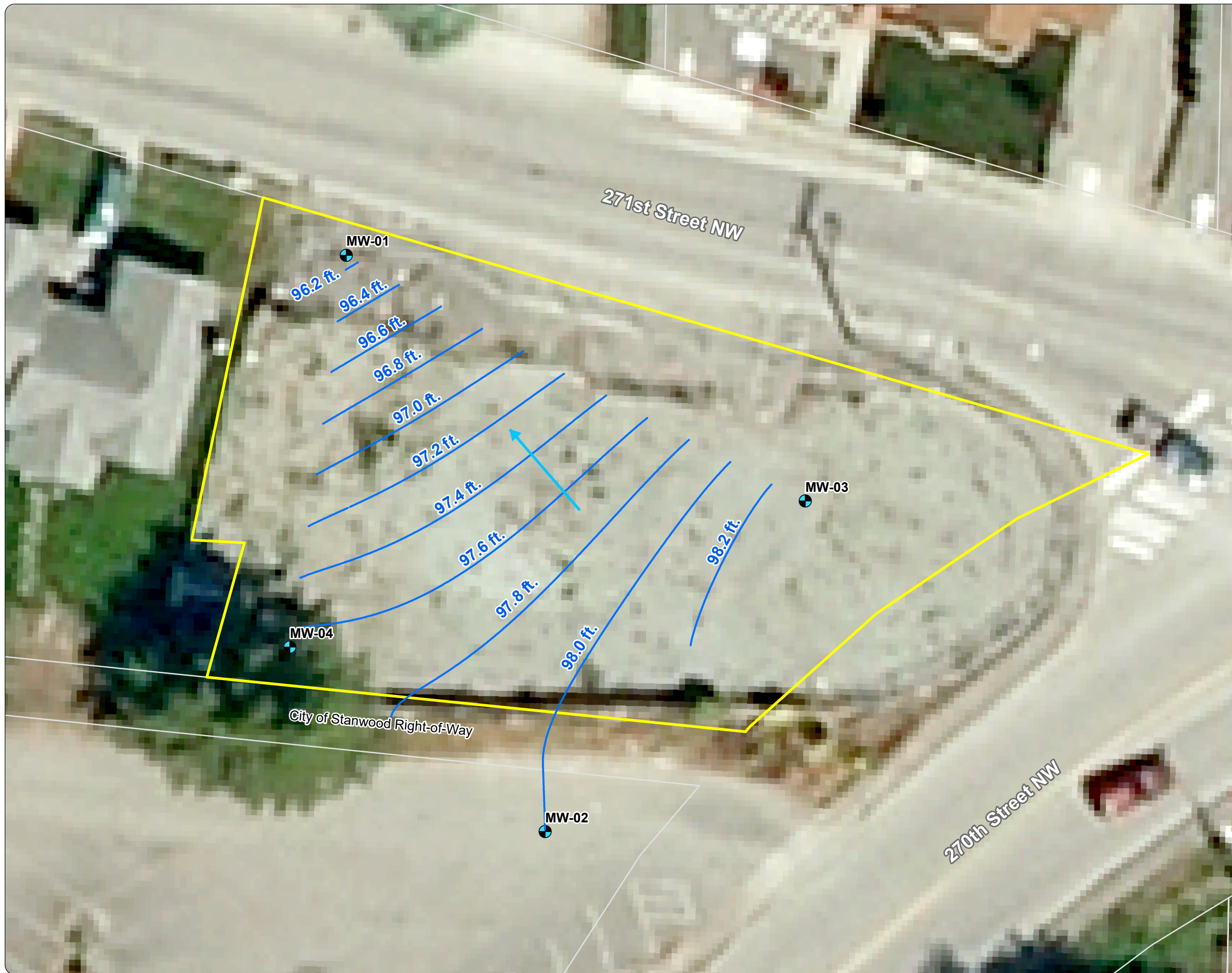
Figure 2-3 Potentiometric Groundwater Contours Raplee Property Stanwood, Washington
