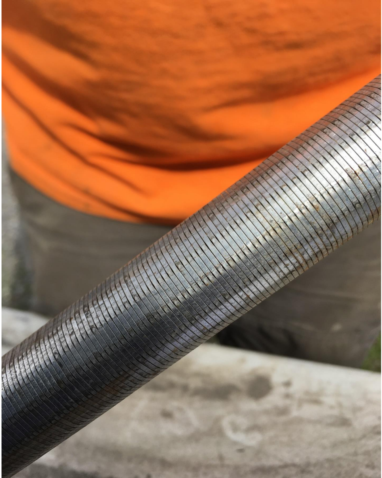
Photograph 3 – Close-up of \frac{3}{4} -inch diameter stainless steel screen (0.010-inch slot size) inserted in borings SB-2 and SB-4 in attempt to obtain groundwater samples for laboratory analyses.
