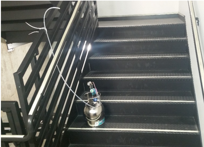
Photograph 7. Indoor air sample IA25, installed in Stairway 1 on Parking Level P1.
