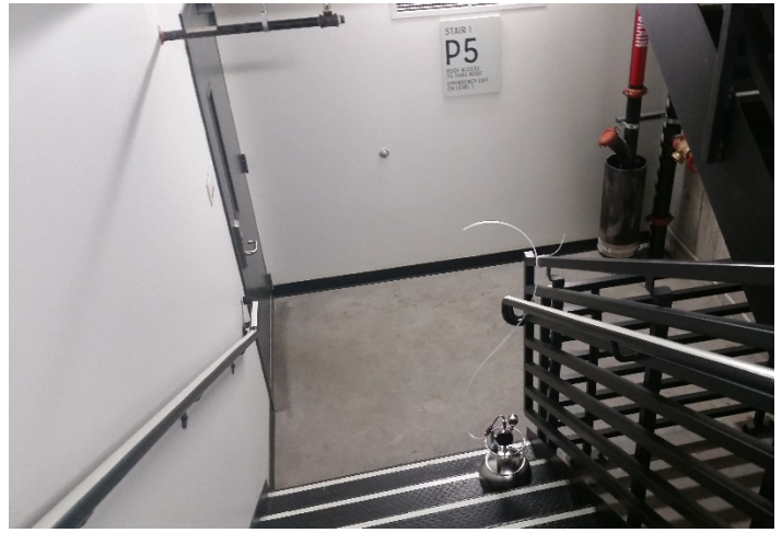
Photograph 4. Indoor air sample IA23, showing sample tubing installed in breathing zone.
