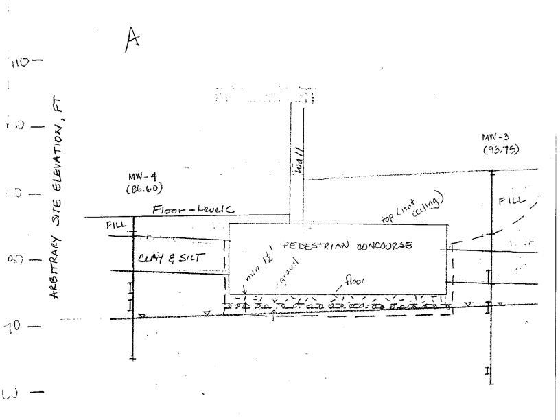
T-1772-02 CROSS SECTION A-A' SHW Fig 4 (2012) PRELIMINARY
