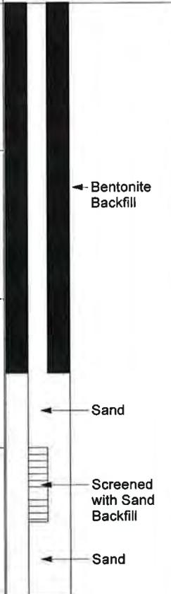
← Bentonite Backfill
