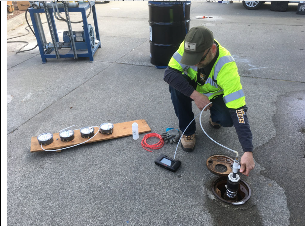
Photo #2: Measuring vacuum at wells prior to startup of the SVE system.
