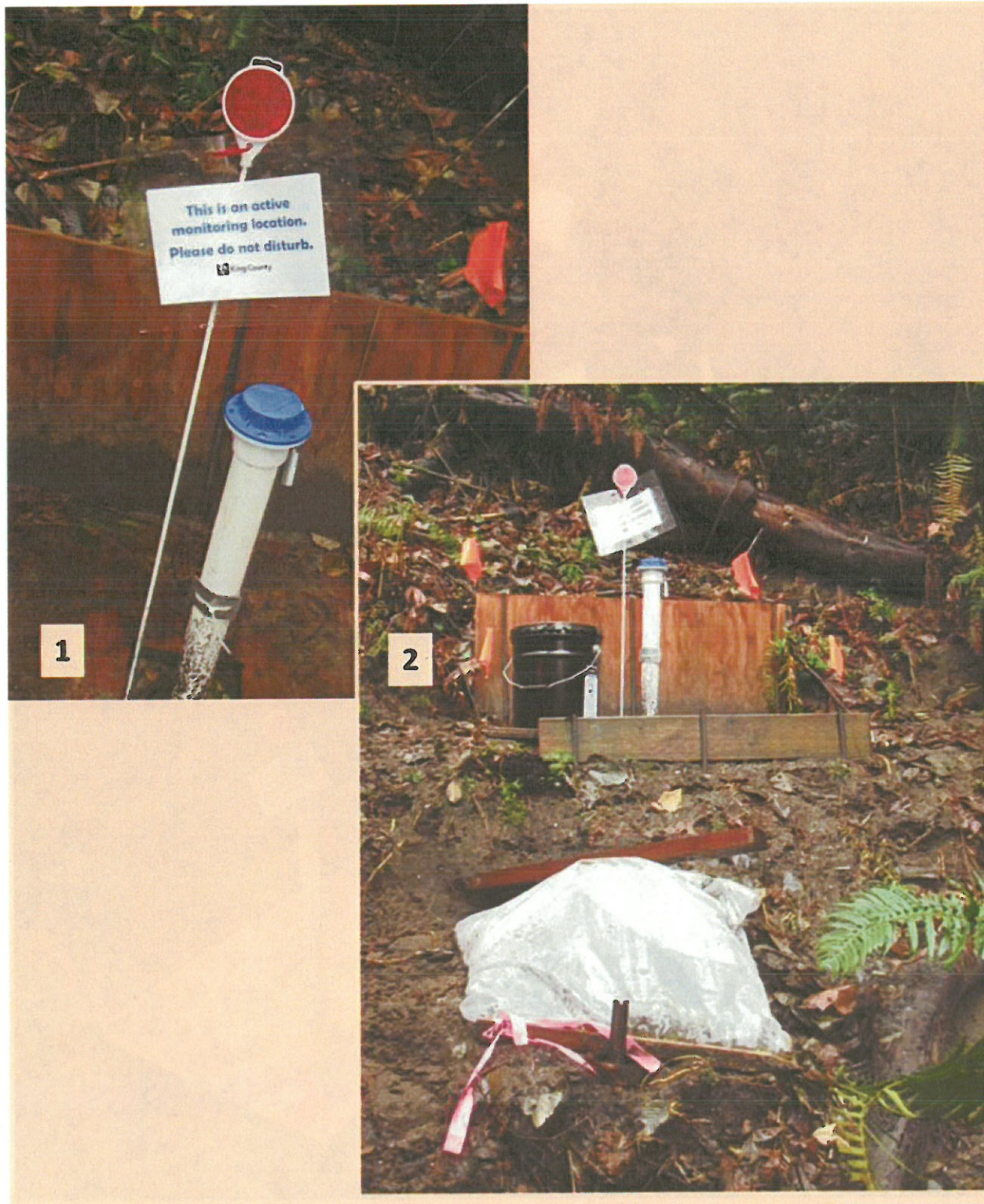
(1 & 2) Well MW-32; DOE Well tag # APJ-048. Pictures show augering platforms, wastewater discharge bucket, and auger sediment cuttings in plastic wrapping. Well is locked with locking caps and locks.
