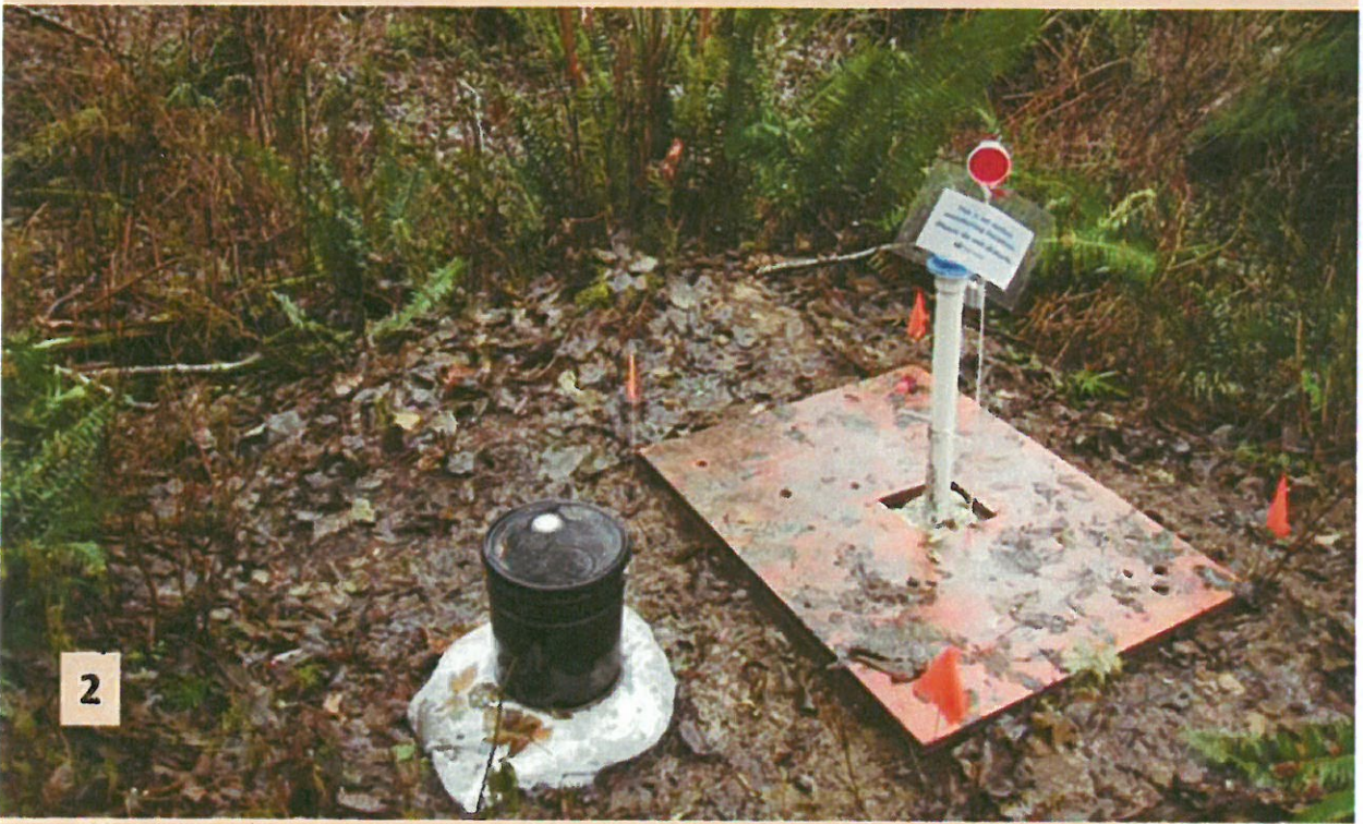
(1) Well MW-30 ; DOE Well tag # APJ-049 (2) Well MW-31; DOE Well tag # APJ-050. Both pictures show augering platforms, wastewater discharge bucket, and auger sediment cuttings in plastic wrapping. Wells are locked with locking caps and locks.
