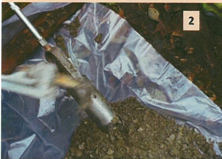
(1) Hand augering through platform access hole (2) Removing coring sediments (3) Saturated sediments in auger bit (4) Driller using soil sampler
