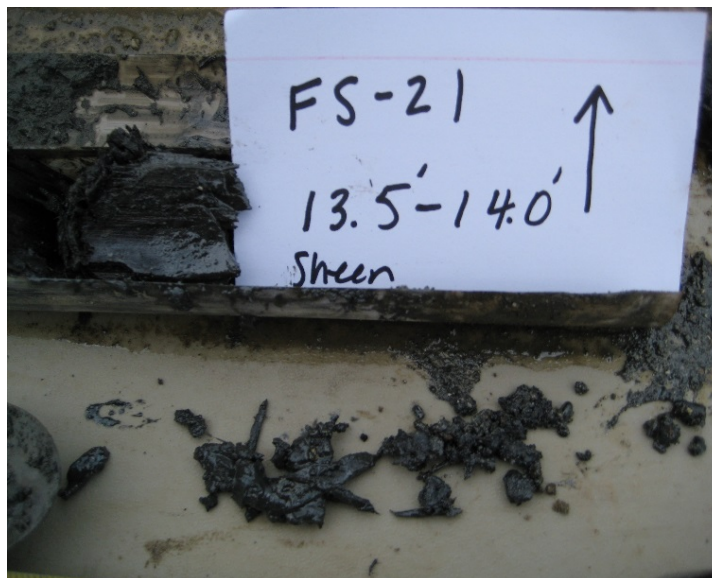
Exhibit 1. Visible wood in FS-21 boring
