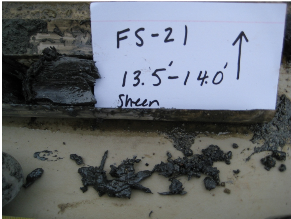
Photograph 9. Soil boring Location FS-21 showing heavy sheen observed from 13.5 feet to 14 feet bgs, January 2013.
