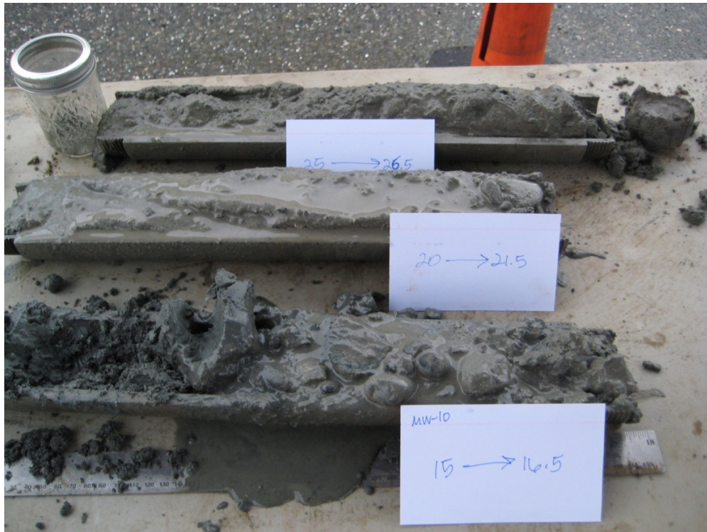
Photograph 11. Split spoons from well installation at Monitoring Well MW-10 in the Northern Shoreline Area, January 2013.
