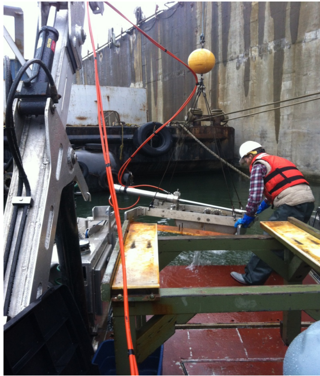
Photograph 15. Power grab sampler collecting nearshore sediment samples, January 2013
