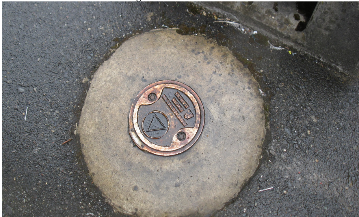
Photo 9: Groundwater Monitoring Well MW-Y
