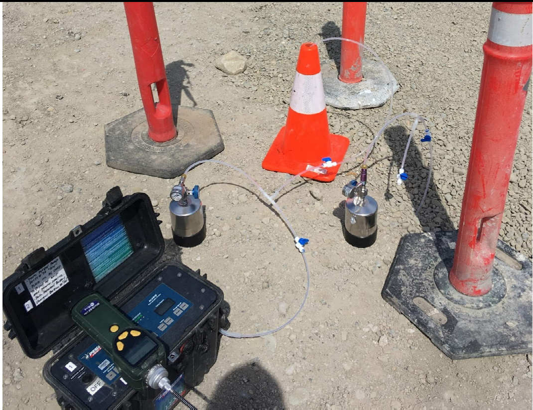
Photograph 9. VOC vapor sampling equipment.
