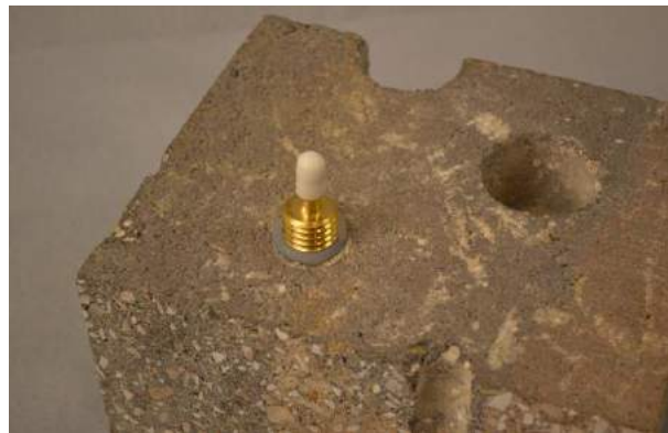
Figure 3. Installed VAPOR PIN®
