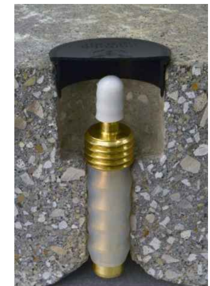
PHOTO - INSTALLED VAPOR PIN
