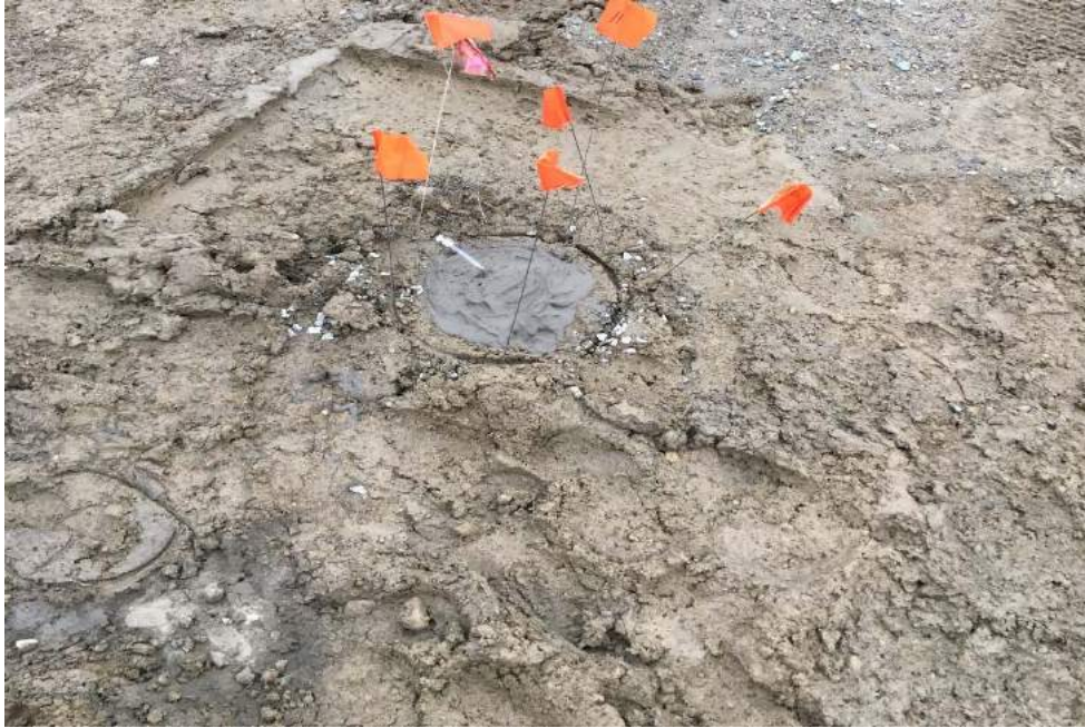
Caption: Capped surface tubing to vapor sample implant
