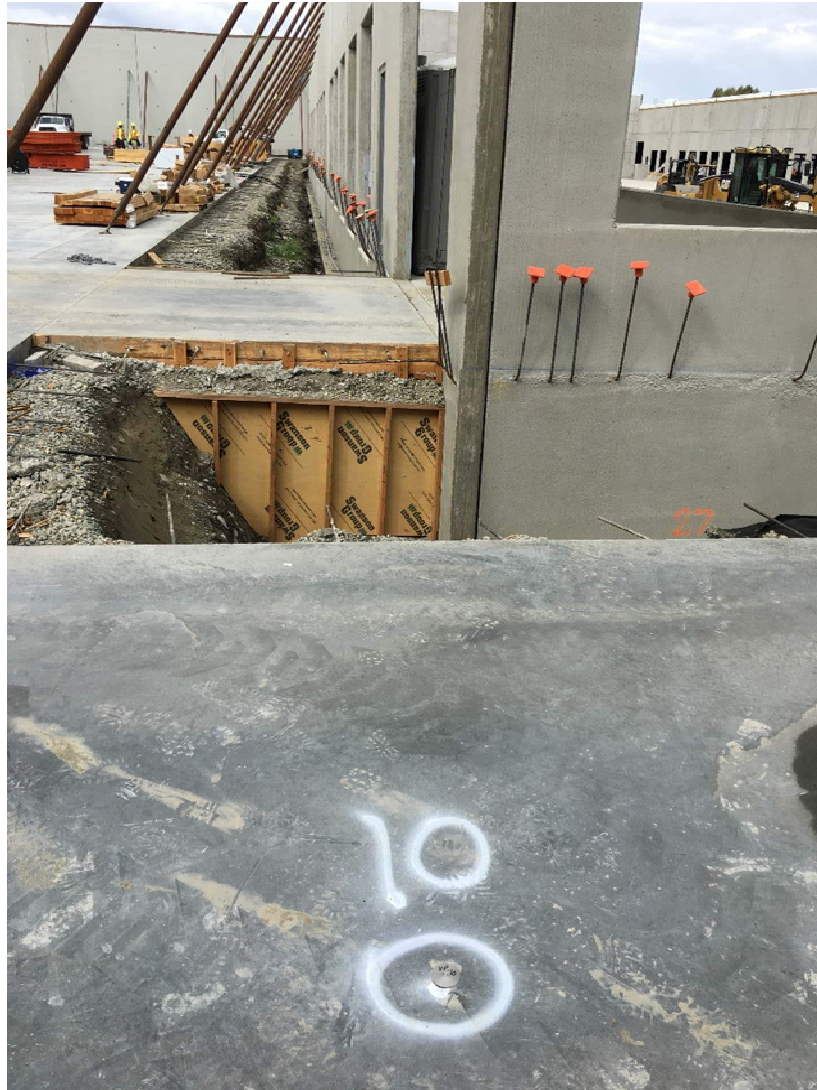
Vapor Pin VP-10 in Ecology adjusted location with stainless-steel cover. VP-10 is adjacent to the northeast office room in Building B. Looking west-northwest
