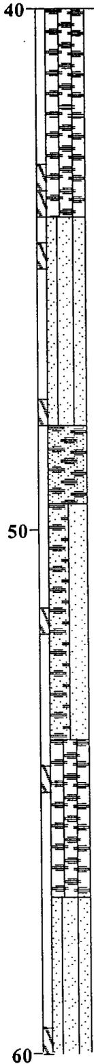
SILTY SAND with gravel and cobbles (SM); olive gray, fine to coarse; some fines; little coarse gravel; dry (STRATIFIED DRIFT)
