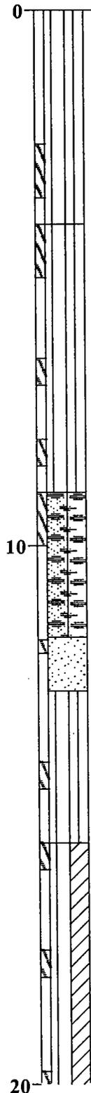
SILT with organics and gravel (ML); moderate brown; abundant roots; trace fine to medium sand; medium to coarse gravel; damp (DISTURBED TILL FILL)
