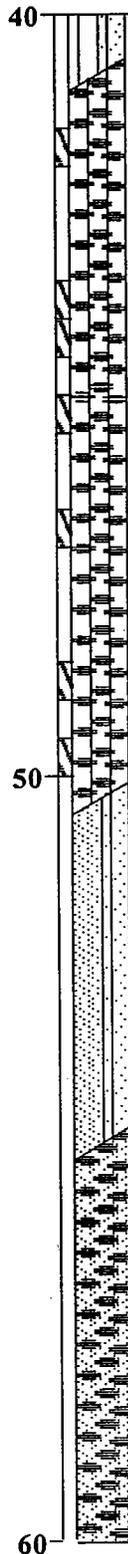
SILTY GRAVEL with sand (GM); light olive gray; mostly fine to medium; occasional coarse gravel beds; some fine to coarse sand; little to some fines; water added (STRATIFIED DRIFT)
