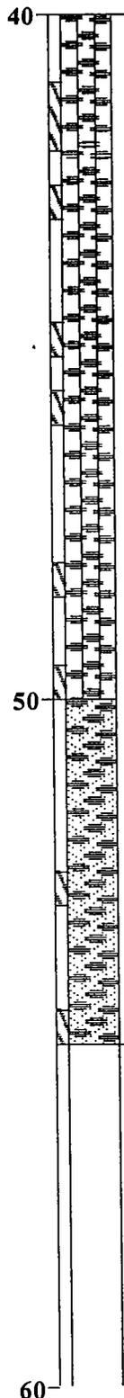
SILTY GRAVEL with sand (GM); medium gray, medium to coarse; some fine to coarse sand; some medium gray fines; adding water to remove cuttings (STRATIFIED DRIFT)
