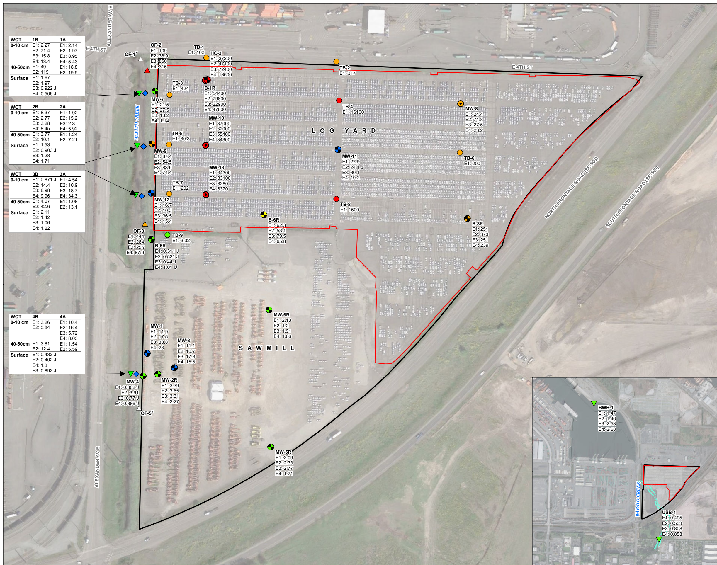
FIGURE 7-3 Arsenic Concentrations in Groundwater, Porewater, Surface Water, and Outfall Discharge - Event 1 through Event 4 Remedial Investigation Report Parcel 15 Tacoma, WA
