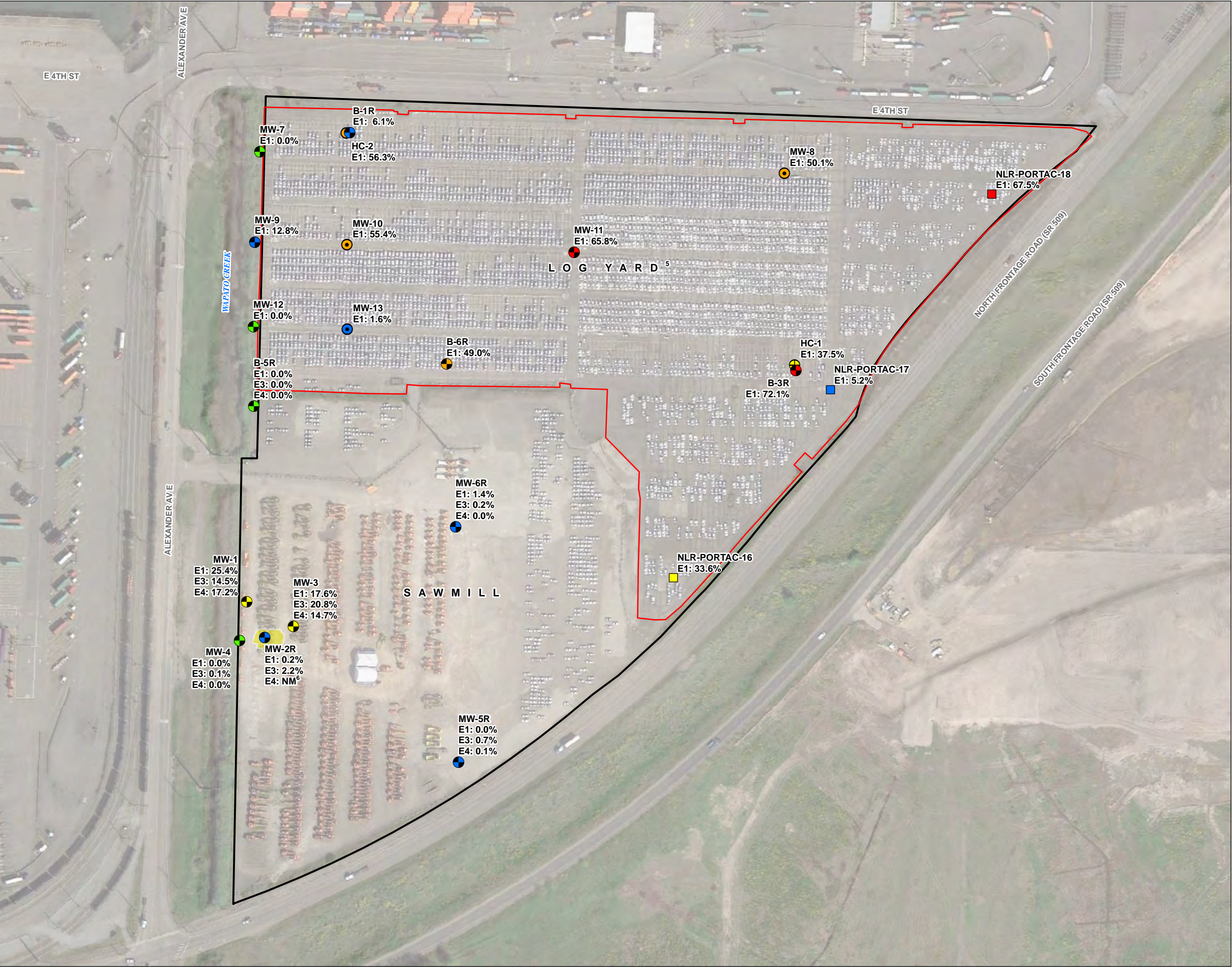
FIGURE 7-4 Methane Headspace Readings - Event 1 through Event 4 Remedial Investigation Report Parcel 15 Tacoma, WA
