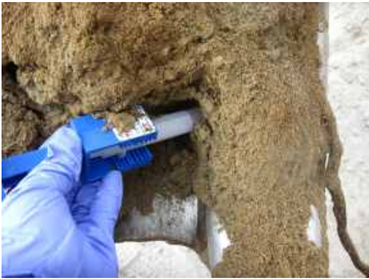
Photograph 03: Soil sample collection - EPA Method 5035
