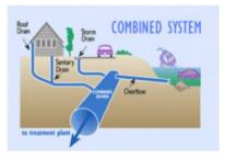
The CSO Project: The city recently bought a five-million gallon tank and 12.5 acres of property from Rayonier. The tank will hold excess stormwater and sewage during very heavy rains. This water will later be treated at the sewage treatment plant. To connect existing stormwater pipes to the tank, the city will install new pipes across the Rayonier property (see map on page 3).
