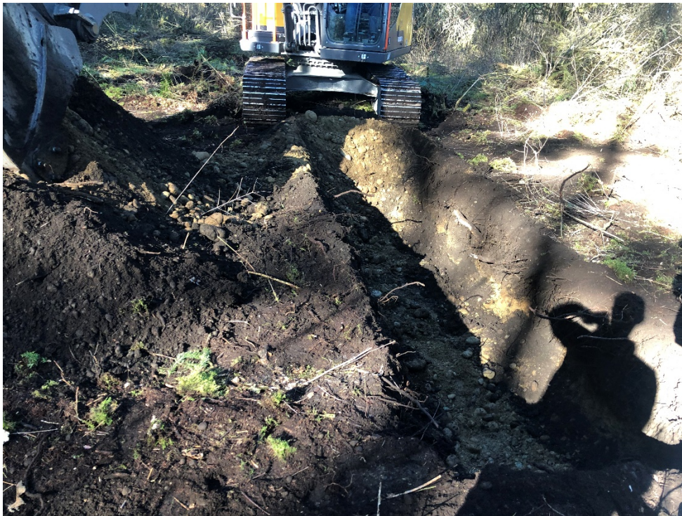
Photograph 4: Excavation of Test Pit 8 (TP-8). Approximately 2feet of brown, poorly graded sand with organics over a foot of weathered outwash over unweathered outwash, extending the bottom of excavation.
