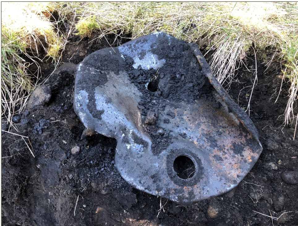
Photograph 8: Steel object uncovered at TP-9. Object appeared to be a drum lid with heavy petroleum odor.
