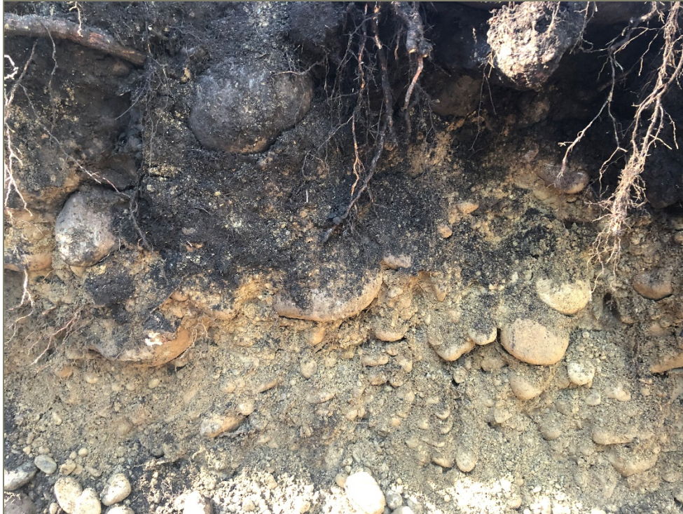
Photograph 5: Transition from brown sand with organics to weathered outwash.
