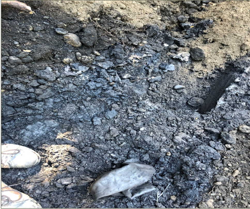
Photograph 7: Rubber tube-tire uncovered at TP-9. Blue-gray soil staining with a pungent petroleum odor.
