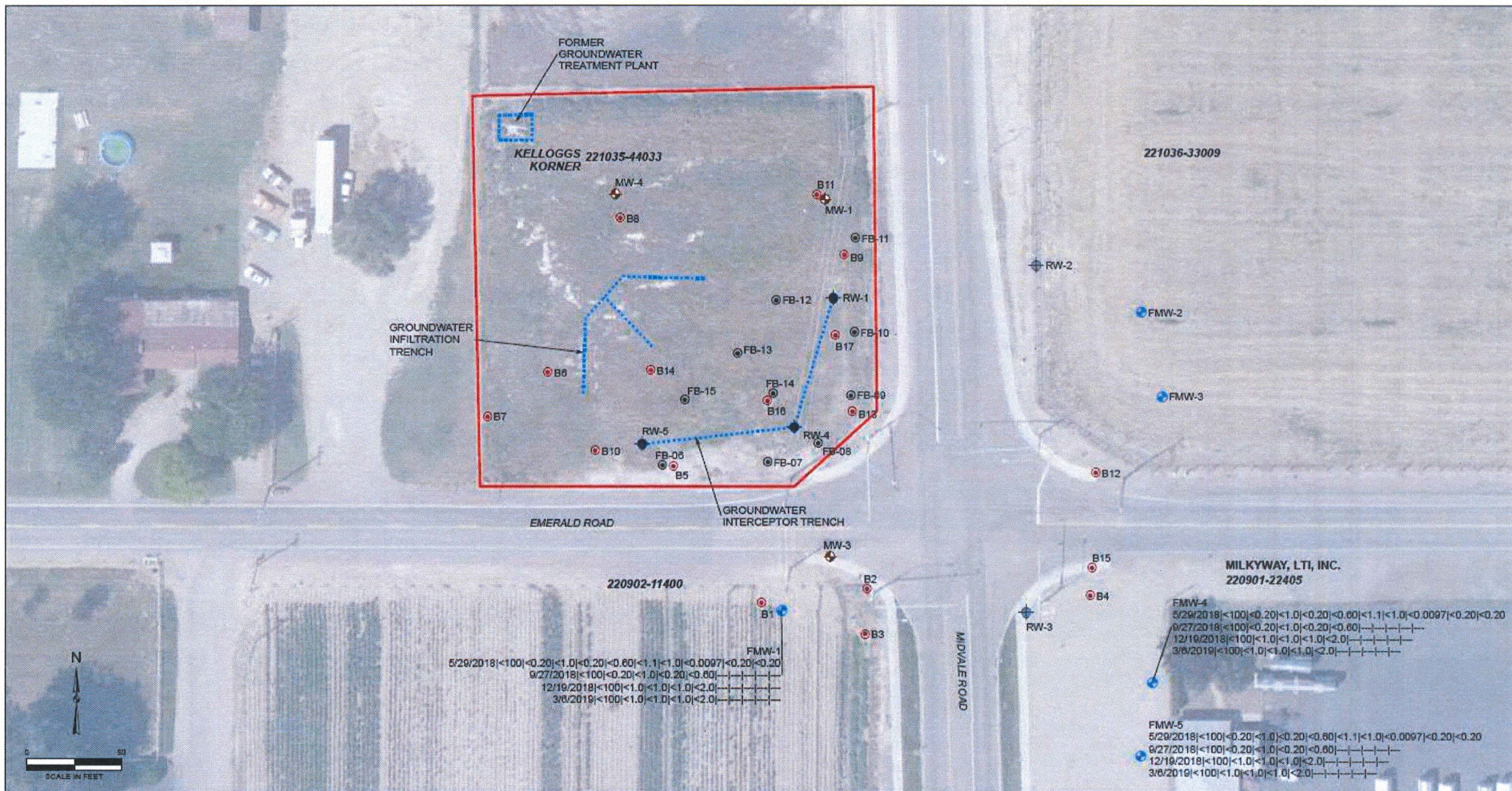
FIGURE 2 SITE PLAN SHOWING GROUNDWATER ANALYTICAL RESULTS KELLOGGS KORNER MIDVALE AND EMERALD ROADS SUNNYSIDE, WASHINGTON FARALLON PN: 1432-001
