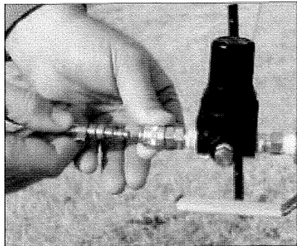
FIGURE 7.6: Attach the foot pump to the pneumatic head using the low-pressure hose with quick connects.
