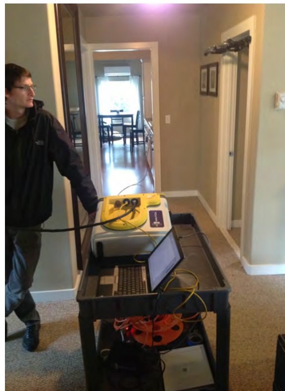
Photograph 4. Using the Hapsite GC/MS to locate indoor sources of the chemicals of concern, November 2012.
