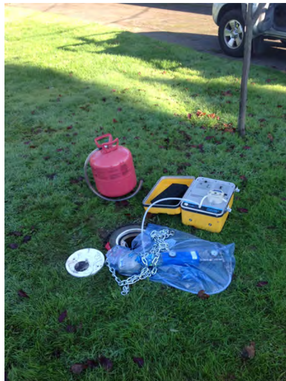
Photograph 14. Soil gas sampling setup, November 2012.
