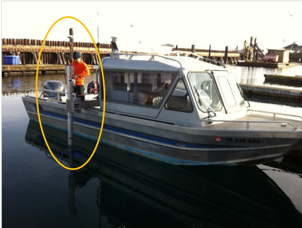
Figure 1. Multi-beam Transducer Pole Mount and Sonar Installed
