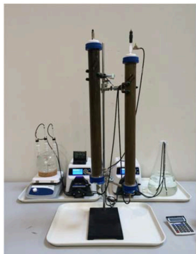
Figure 9. o-Xylene column study set-up.
