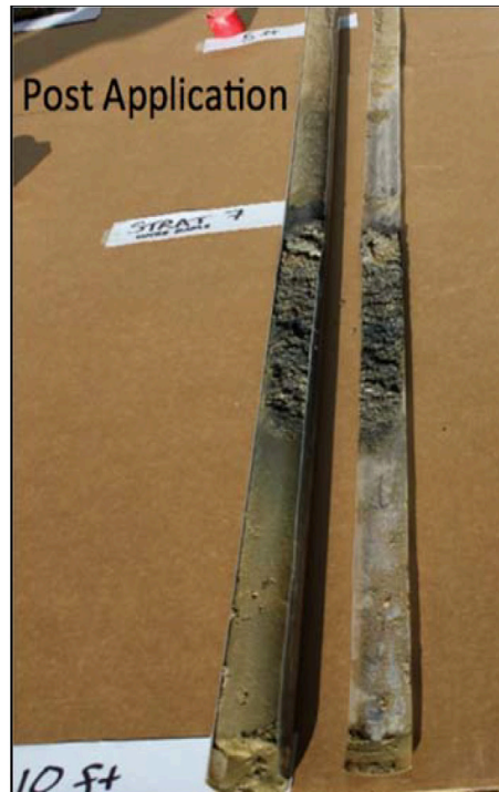
Figure 22. Post-Application Soil Core
