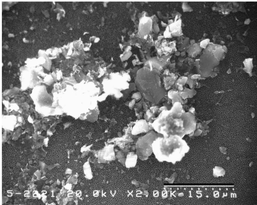
Figure 3. Photomicrograph of aluminum oxide filter surface with particles found on sub-sample B. Scale bar is 15 micrometers in length.
