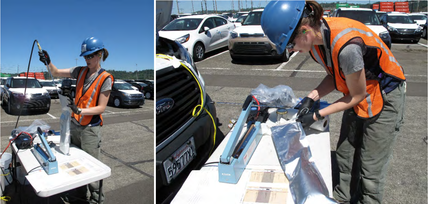
Photo E-16: Sealing soil sample cores anoxically in nitrogen purged Mylar bags containing oxygen absorbers.
