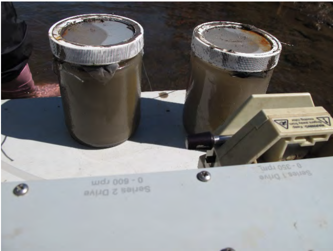
Photo E-21: Comparison of NMDS turbidity using the 120 micron nylon mesh (left) and the 22 micron mesh (right)
