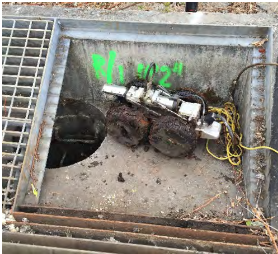
Photo E-9: Stormwater video camera (left) and an image looking upgradient at the spill containment vessel near manhole #1 (right).
