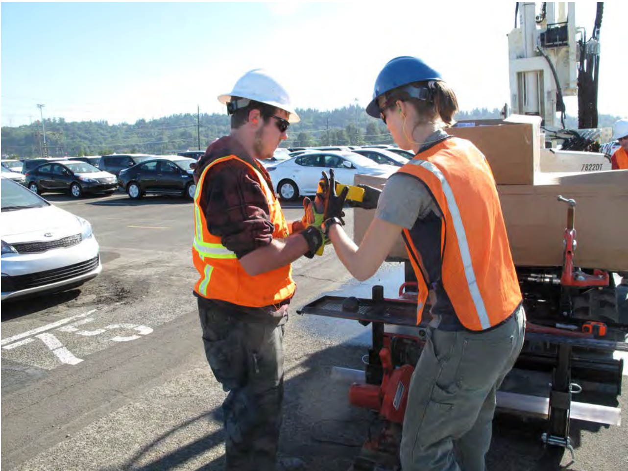
Photo E-15: Sealing soil samples in clear Geoprobe liner
