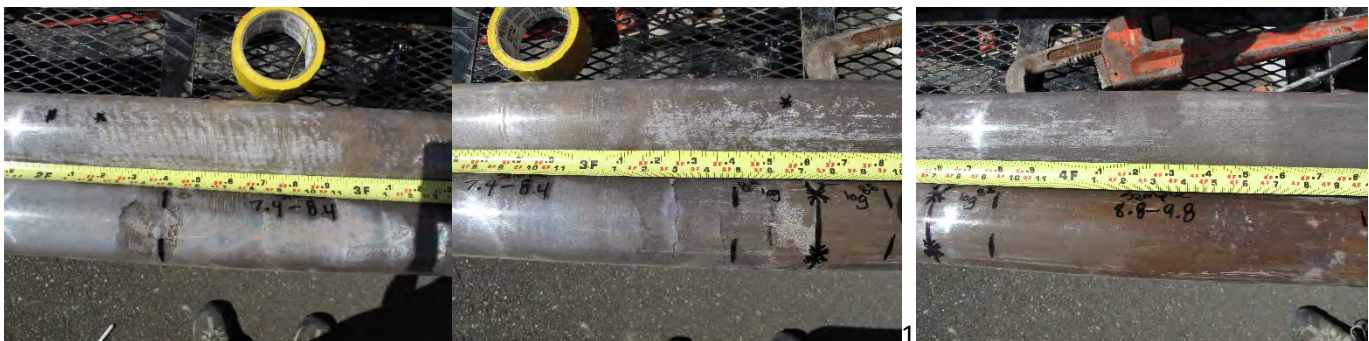
Photo E-5: TB-9: A different colored (dark brown to reddish brown) poorly graded sand with rootlets, observed from 2.4 to 5 ft bgs could be evidence of the former drainage ditch, but no obvious fine-grained channel bed was observed so the unit could also just be fill material (Photo E-X). Sample was collected for archival from 2.4 to 3.4 ft bgs. Unit is underlain by the more typical dark gray poorly graded sand, indicative of the hydraulic dredge fill unit, from 5 to 7.4 ft bgs.
