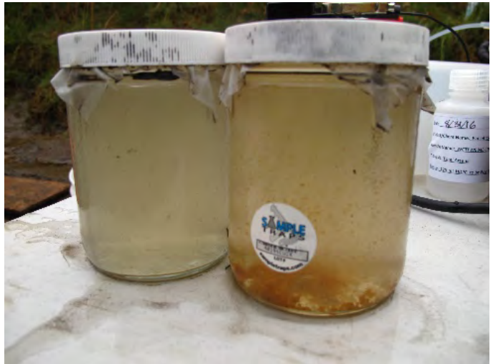
Photo E-21: Comparison of NMDS turbidity using the 120 micron nylon mesh (left) and the 22 micron mesh (right)
