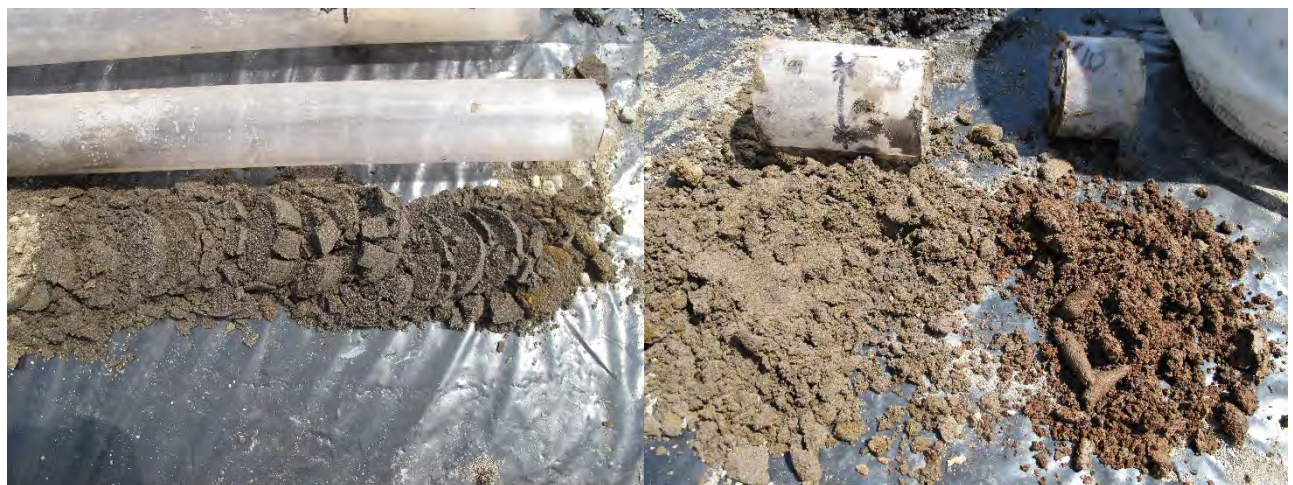
Photo E-6: TB-9: Apparent contact at 7.4 feet bgs between the distinctive upper poorly graded fine-grained sand (hydraulic fill) above and a fine-grained channel bed and/or overbank deposits below, with interbedded reddish brown clay, sand and silt deposits observed between 7.4 and 12 feet bgs. Soil samples were collected and analyzed from above (7.4 to 8.4 ft bgs) and below (8.8 to 9.8 ft bgs) this contact. This unit is suspected to constitute the Wapato Creek channel alignment observed through the 1950's (Appendix A.1).
