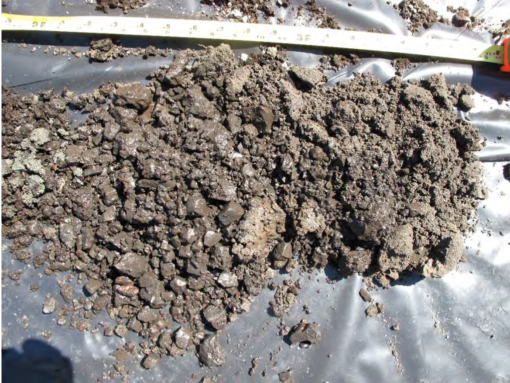
Photo E-3: Saturated slag gravel layer at base of Fill Containing Slag (as observed in MW-13)
