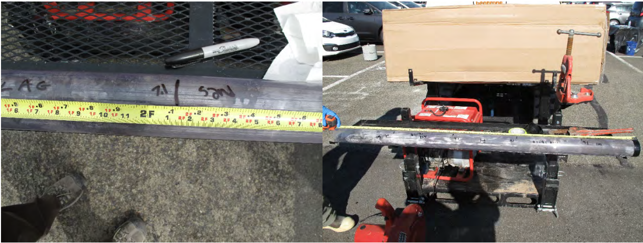
Photo E-14: Marking contacts on clear Geoprobe liner prior to cutting sampling intervals
