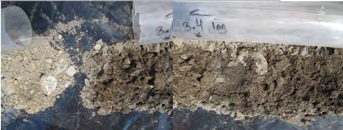
Photo E-5: TB-9: A different colored (dark brown to reddish brown) poorly graded sand with rootlets, observed from 2.4 to 5 ft bgs could be evidence of the former drainage ditch, but no obvious fine-grained channel bed was observed so the unit could also just be fill material (Photo E-X). Sample was collected for archival from 2.4 to 3.4 ft bgs. Unit is underlain by the more typical dark gray poorly graded sand, indicative of the hydraulic dredge fill unit, from 5 to 7.4 ft bgs.
