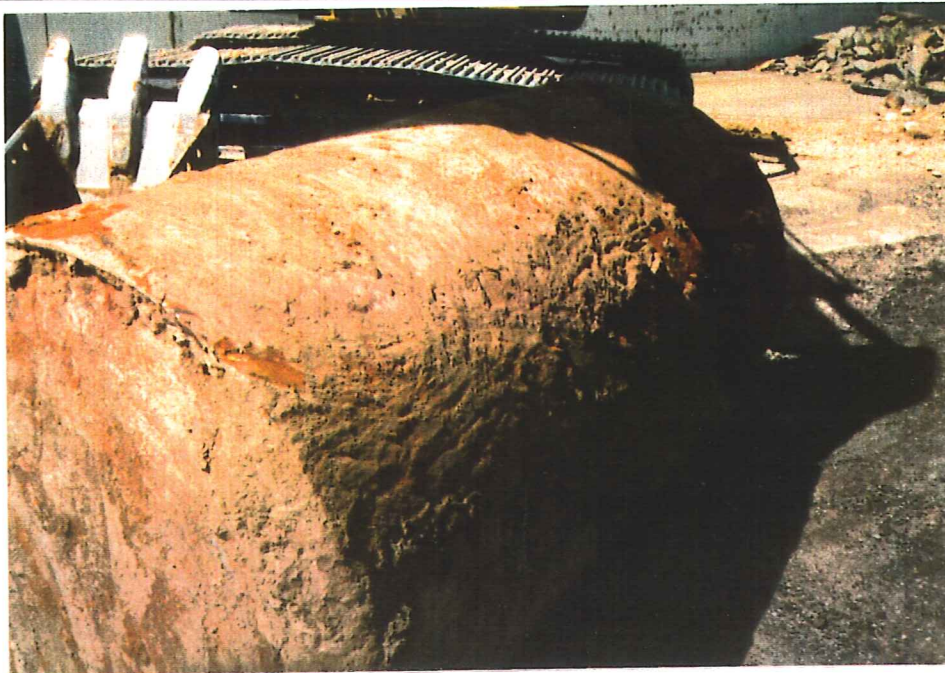
PHOTOGRAPHED BY: Paul Danielson DATE: 8/23/93 VIEW: Bottom of Tank #30. Rust and slight pitting visible. No perforation or stains observed.
