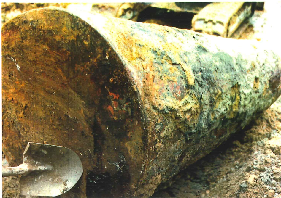
PHOTOGRAPHED BY: Dan Uldall DATE: 8/16/93 VIEW: Tank #10 with staining, rust and pitting on bottom. Removed from south side of 1398 Jadwin Avenue.
