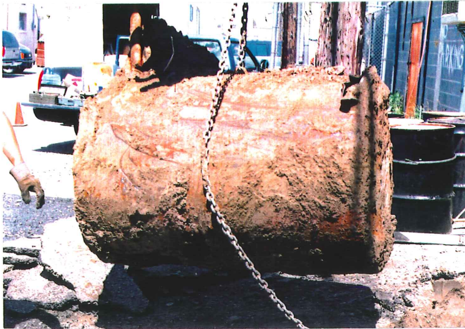
PHOTOGRAPHED BY: Dan Uldall DATE: 8/10/93 VIEW: Tank #4 with rust and pitting on bottom.
