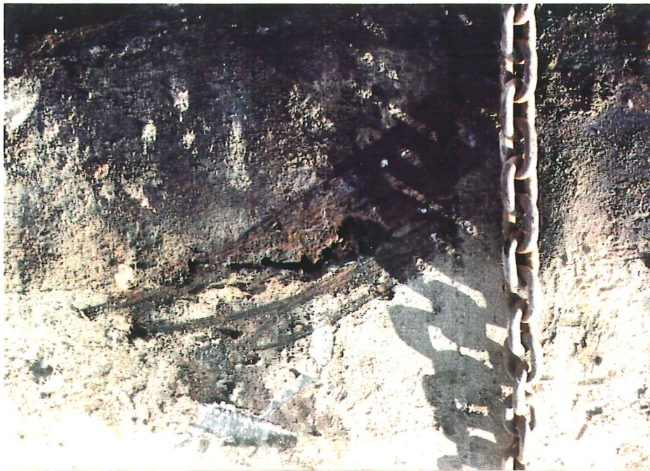
PHOTOGRAPHED BY: Dan Uldall DATE: 8/30/93 VIEW: Rust and perforations visible on bottom of Tank #25.
