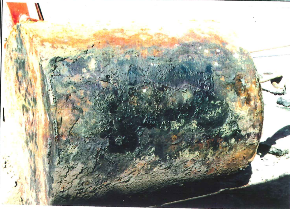
PHOTOGRAPHED BY: Dan DATE: 8/11/93 VIEW: Tank #8 with visible rust, pitting, staining and leakage on bottom.
