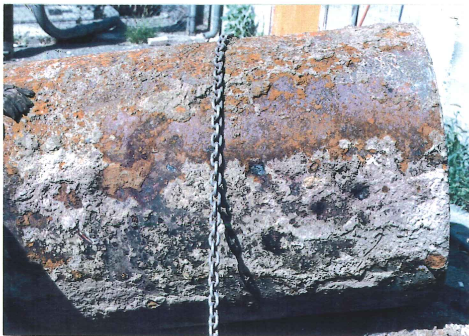
PHOTOGRAPHED BY: Dan Uldall DATE: 8/10/93 VIEW: Rust, pitting and staining visible on bottom of Tank #5.
