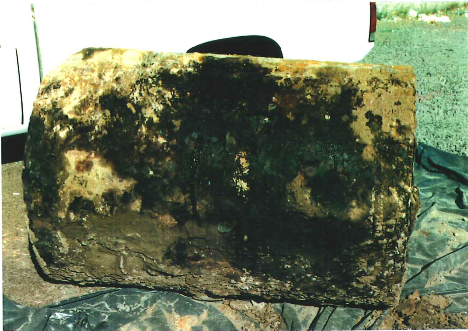
PHOTOGRAPHED BY: Dan Uldall DATE: 8/11/93 VIEW: Rust, pitting and leakage visible staining on bottom of Tank #6.
