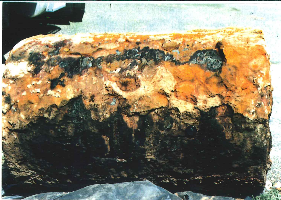
PHOTOGRAPHED BY: Dan Uldall DATE: 8/10/93 VIEW: Rust and pitting on bottom of Tank #2.
