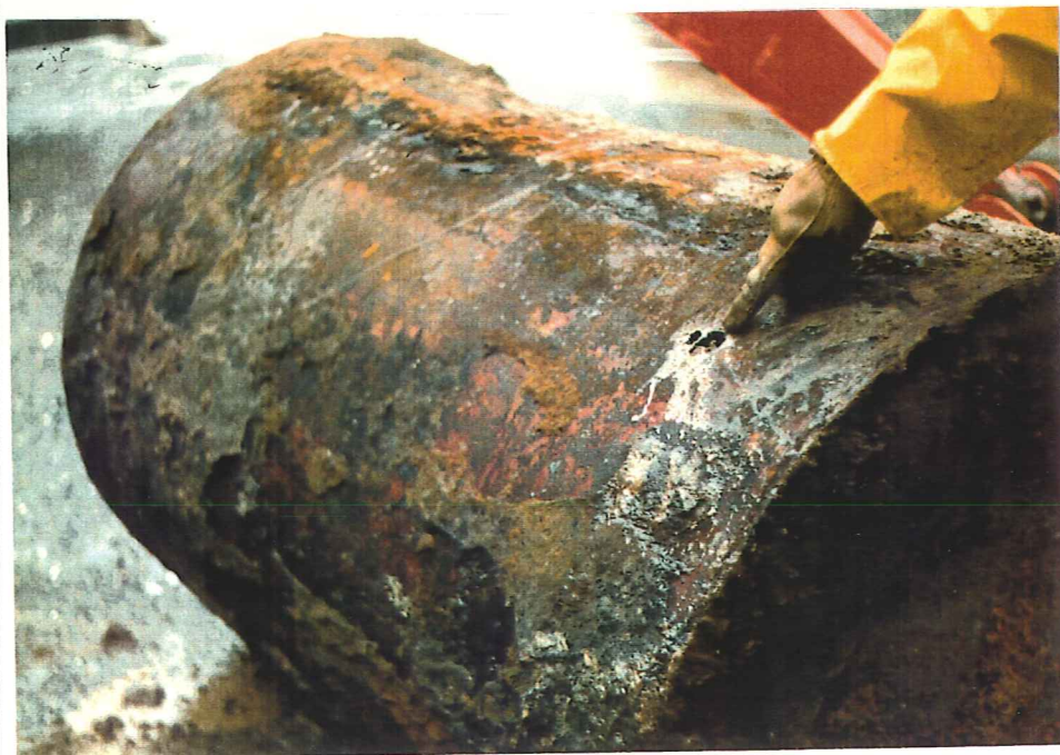
PHOTOGRAPHED BY: Dan Uldall DATE: 8/16/93 VIEW: Tank #13 showing rust, staining, pitting and perforations on bottom. Removed from north side of 1386 Jadwin Avenue.
