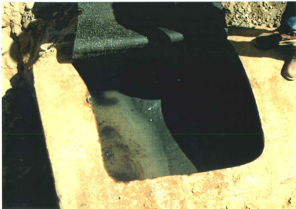
PHOTOGRAPHED BY: Dan Uldall DATE: 8/12/93 VIEW: Contents of Tank #7 as observed after opening access hole. Small amount of residual fuel visible at left after fuel was previously pumped. Remainder of material consists mostly of saturated sandy PCS.
