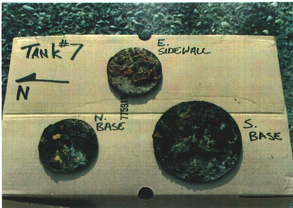
PHOTOGRAPHED BY: Dan Uldall DATE: 8/13/93 VIEW: Condition of Tank #7 exterior at sample locations. Base of tank appears rusted stained and pitted.
