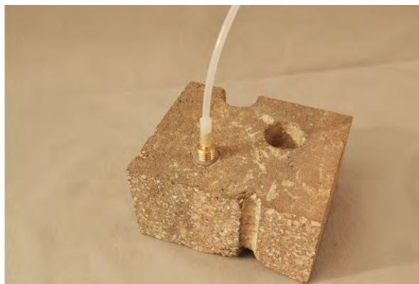
Figure 5. Vapor Pin™ sample connection.
