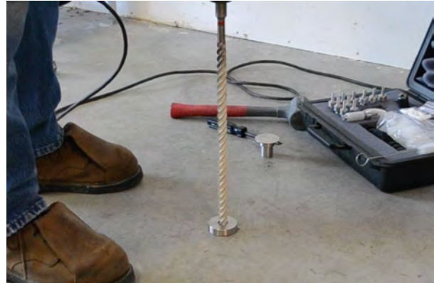
Figure 4. Using the Drilling Guide.
