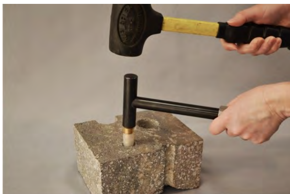
Figure 2. Installing the Vapor Pin™.
