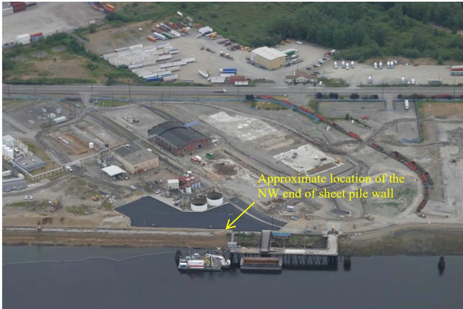
**Photo P-1a (07-02-2004):** Sheet pile wall on the former Arkema site starts just to the southwest of the dock on the site and extends for approximately 900 feet along the bank of the Hylebos Waterway.
