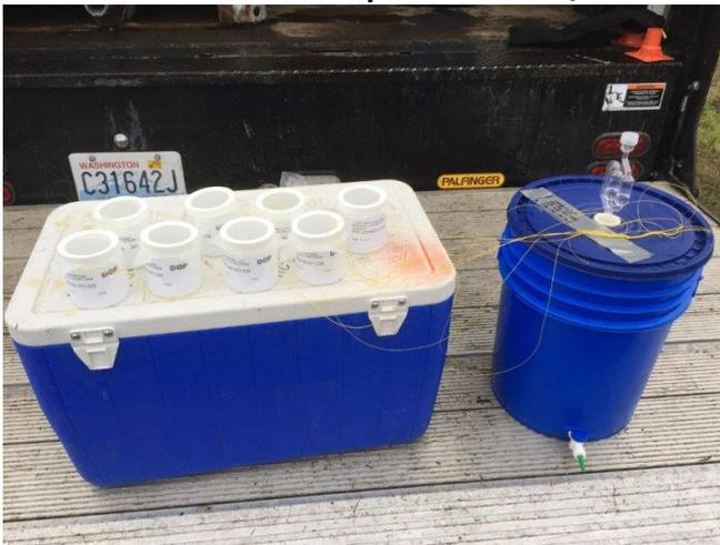
To deploy each pore water NSDS, a shallow trench was excavated at the target location with a decontaminated non-metal hand trowel in order to minimize disturbed sediment. The NSDSs were placed in the small trench, targeting approximately 0 to 10 centimeters
