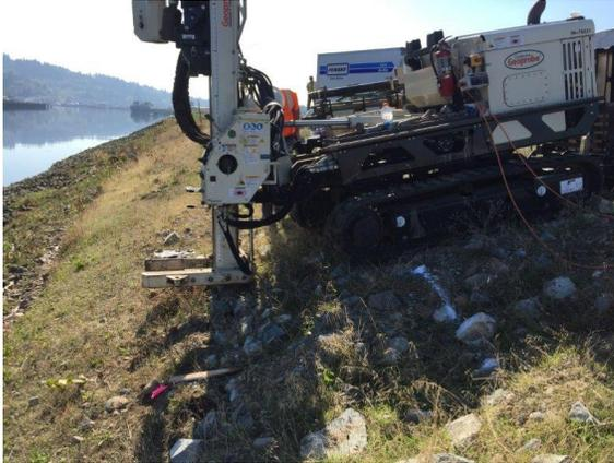
Soil samples were collected directly from within the acrylic core liner using decontaminated stainless steel spoons. Field screening included at least one soil sample for XRF field screening every 2.5 feet of depth at each sampling location.
