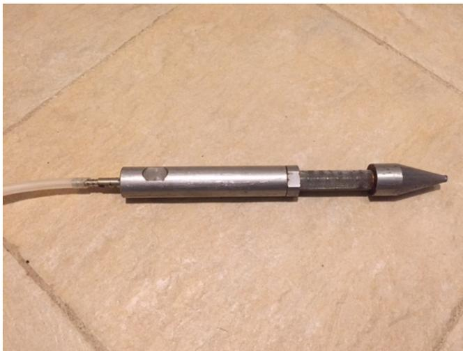
Once the diver seated the sampler into the surface sediment/cap and retracted the probe to expose the screen, pore water was purged by pumping at a rate of 100-500 ml/min. Approximately two to three gallons were purged prior to sampling. Field measurements were made and recorded during the purging for pH, electrical conductivity, temperature, dissolved oxygen (DO), oxidation/reduction potential (ORP), and turbidity. Field measurements were monitored using:
