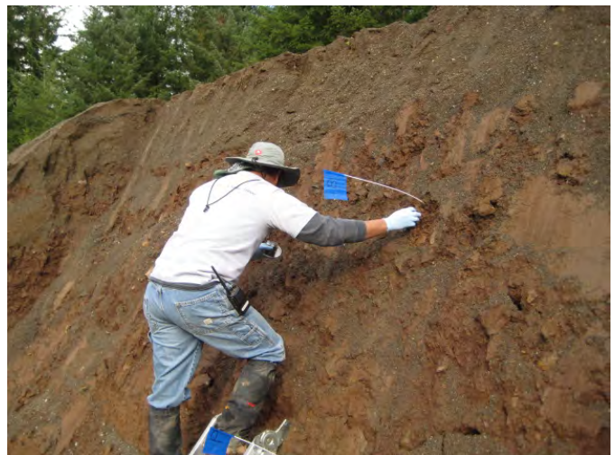
Confirmatory performance sampling on berm face
