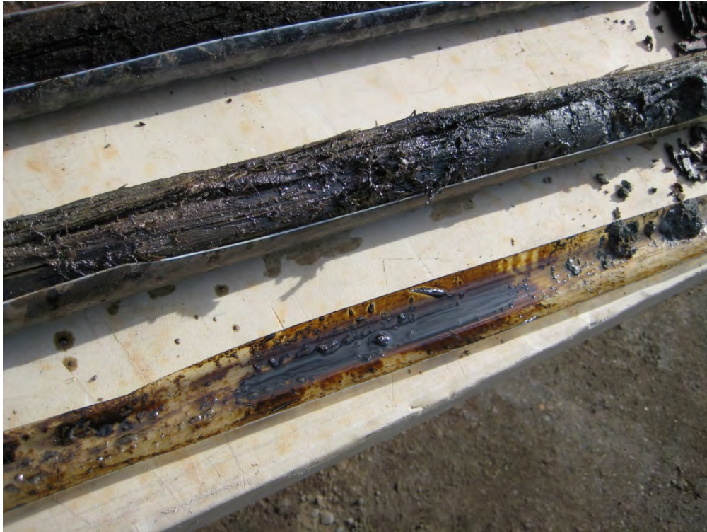
Photograph 3. Soil boring location FS-09a showing creosote-coated piling with heavy non-aqueous phase liquid (NAPL) throughout.
