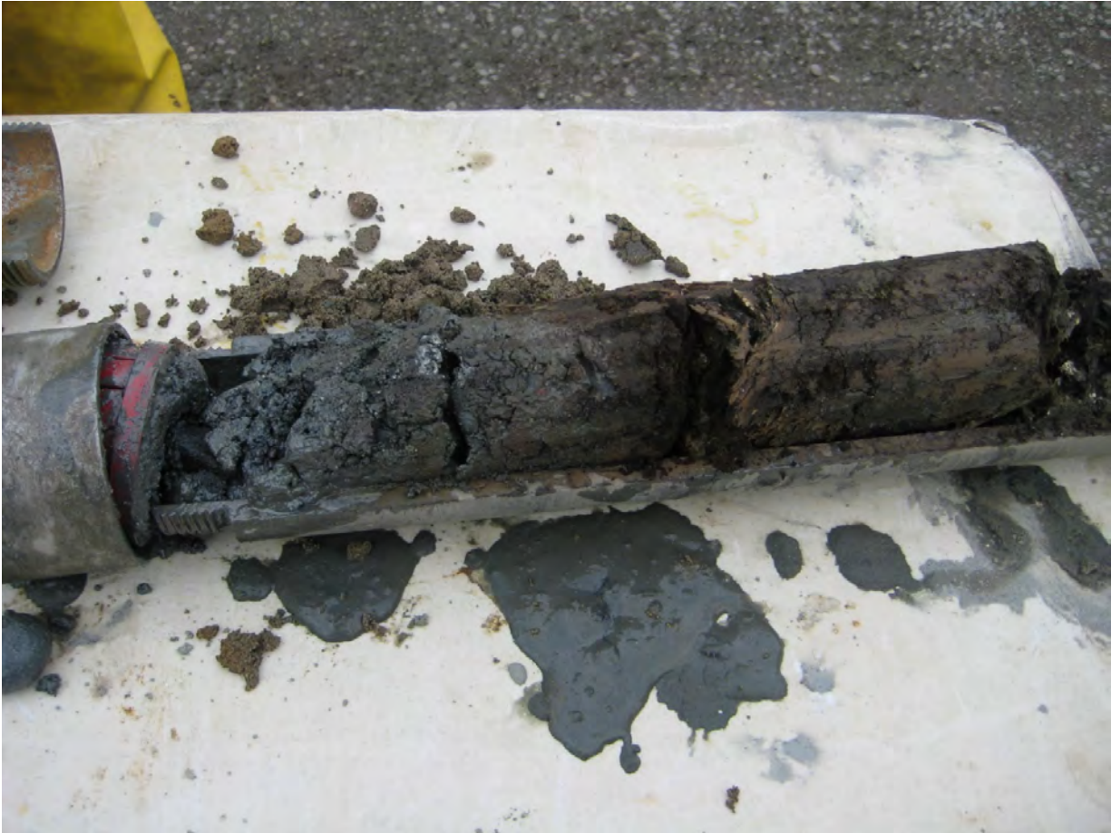
Photograph 5. Split-spoon soil sample taken at MW-09 from 8 to 9.5 feet bgs.
