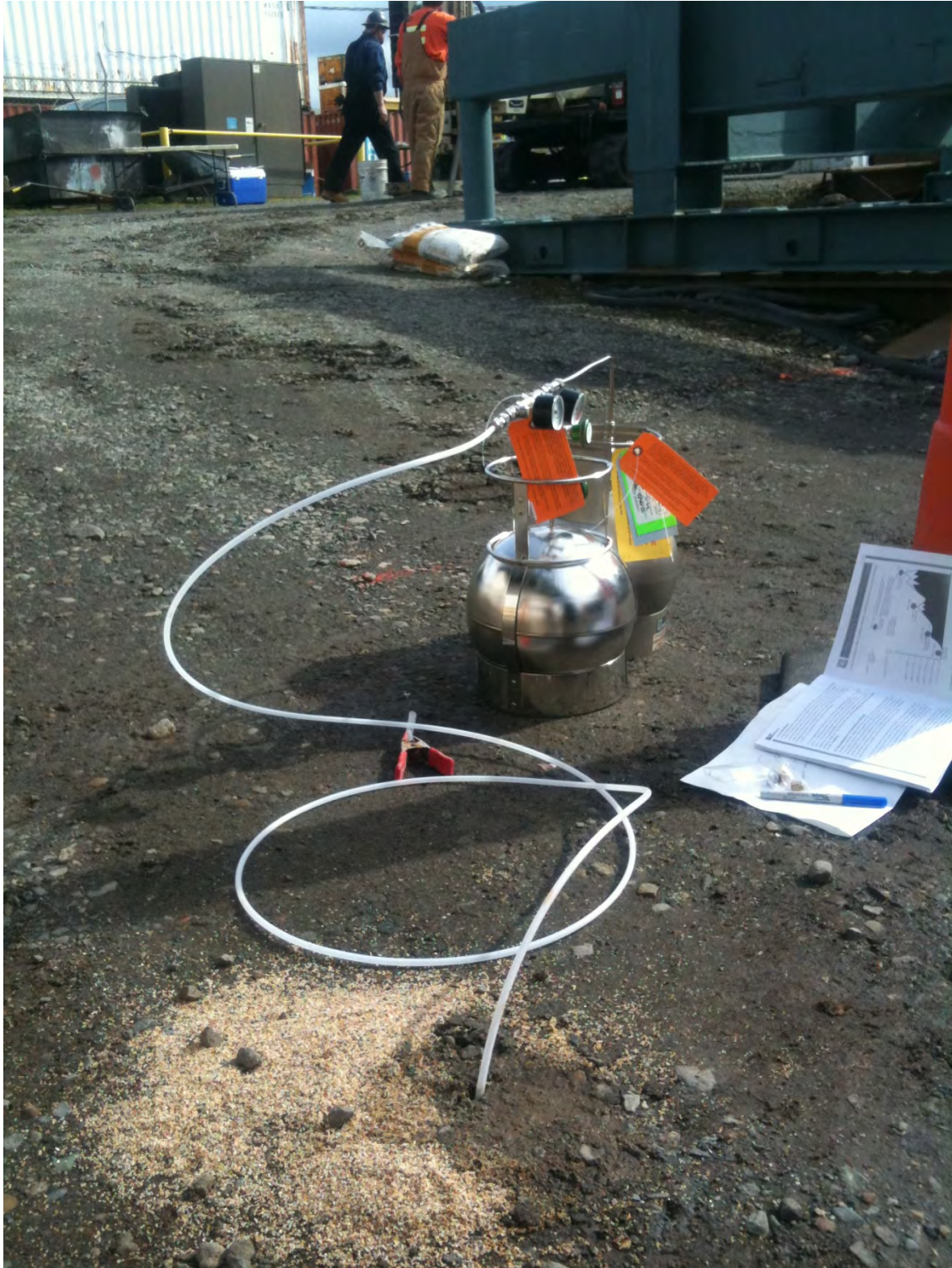
Photograph 6. Soil gas sample set-up at MW-09 at 3.5 feet bgs.
