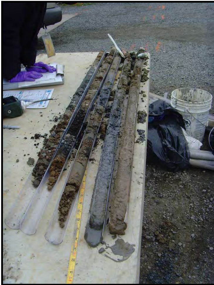
Figure 5. Overview of FS-15 soil samples, showing the layers of fill overlying potentially dredged and finally possibly intact native sediments at the base. The samples are oriented from left (uppermost sample) to right (lowermost sample), with the upper limit of each sample located towards the viewer.
