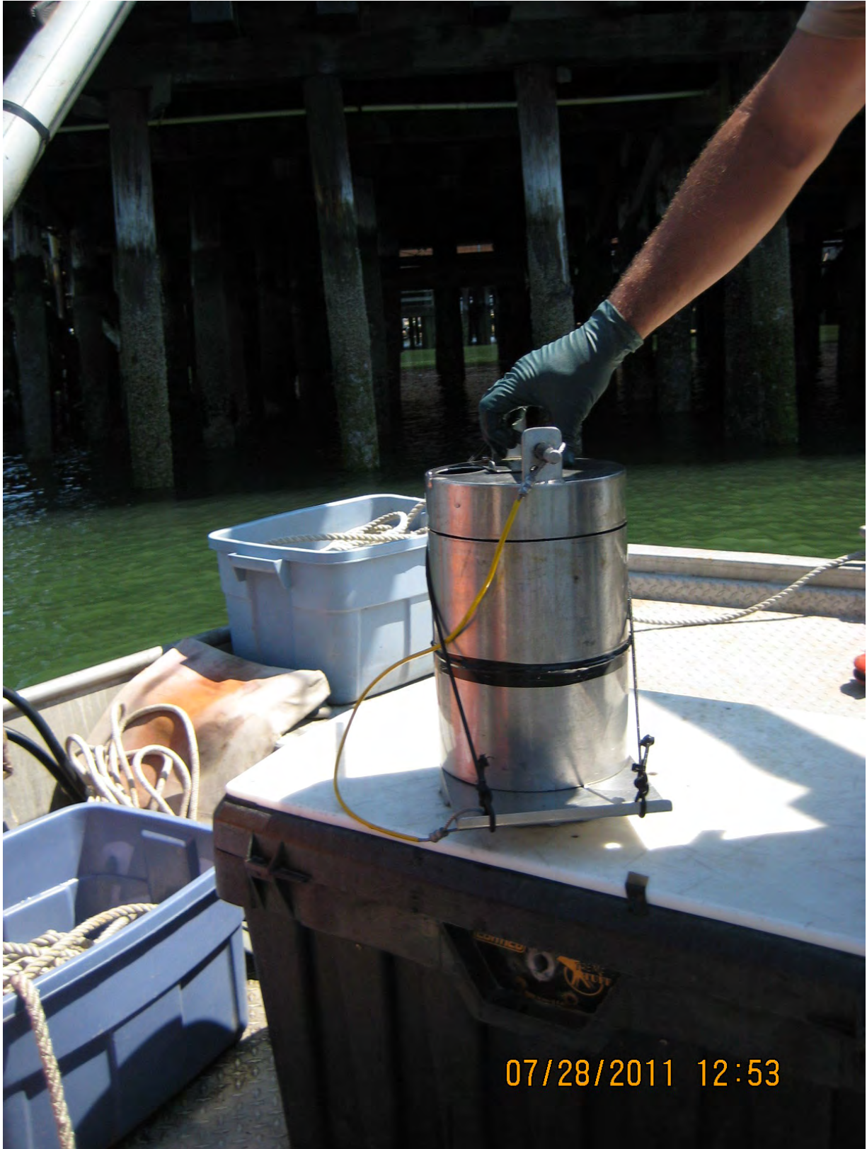
Photograph 10. Diver assisted hand corer used to collect nearshore sediment contingency samples.
