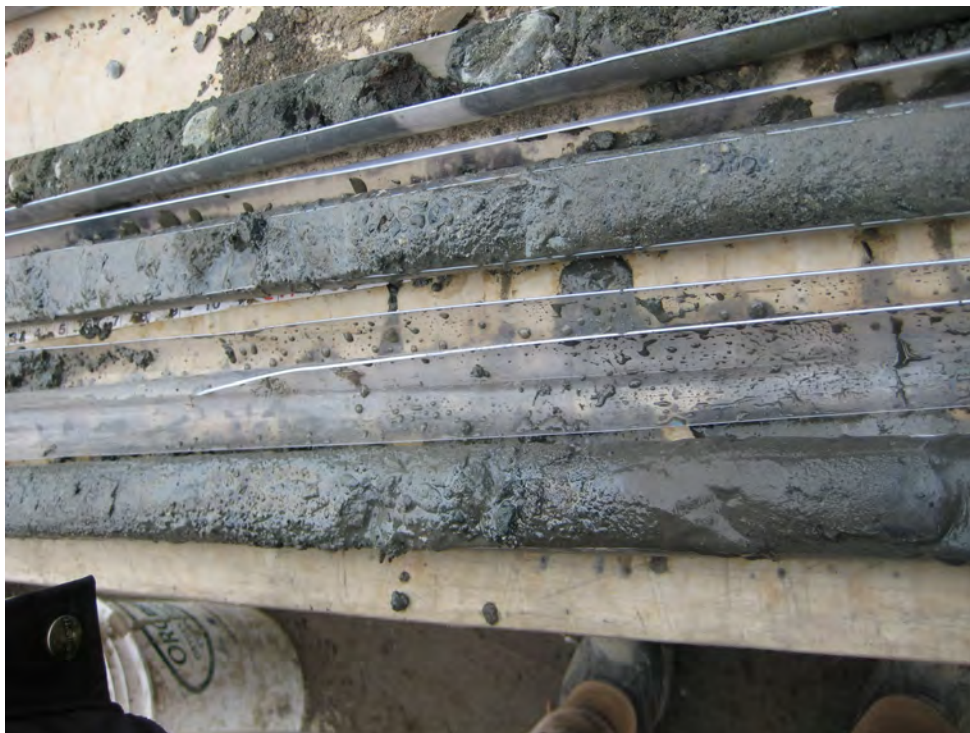
Photograph 2. Soil boring location FS-09 showing heavy sheen observed from 8.5 feet down to 17 feet bgs.
