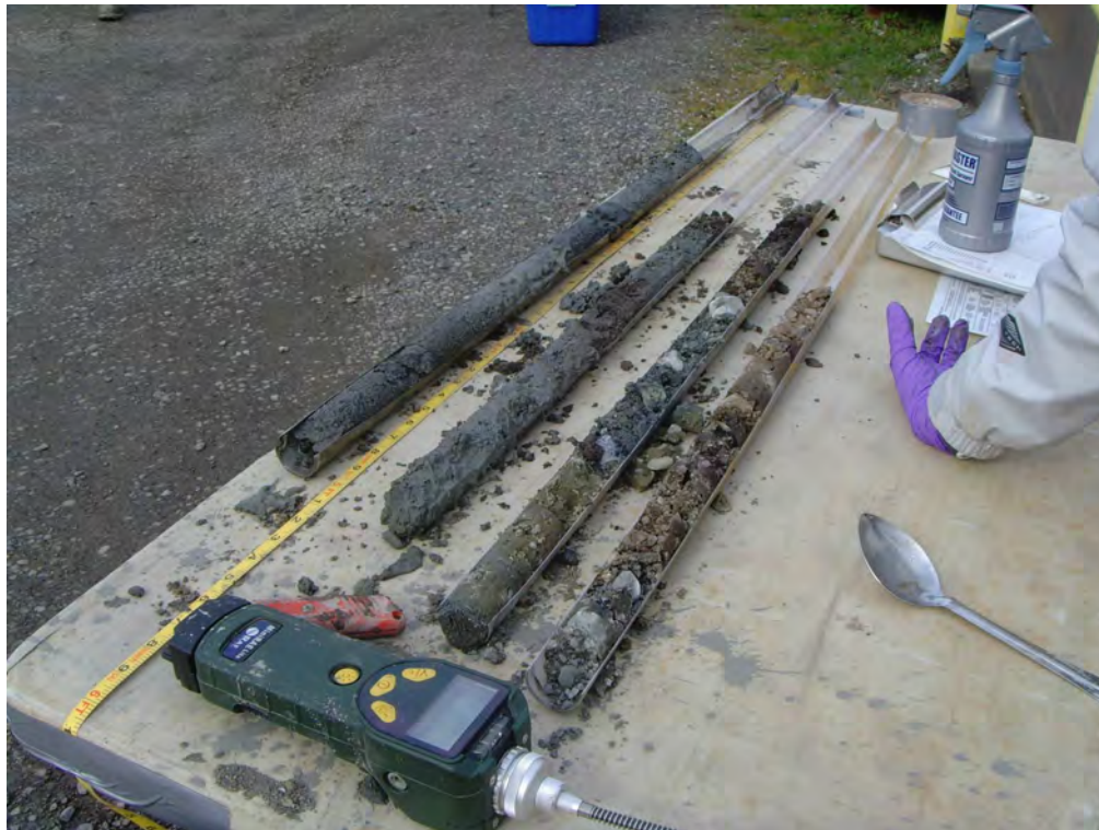
Photograph 1. Soil boring location FS-01 from 0 to 20 feet below ground surface (bgs) showing fill down to native sands.
