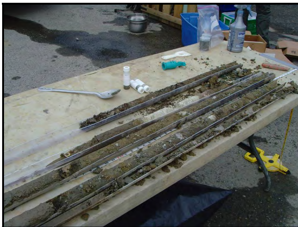
Figure 8. Overview of possible concrete foundation layer observed in FS-14, approximately 6 ftbs (pale gray to white layer in second tube from left).
