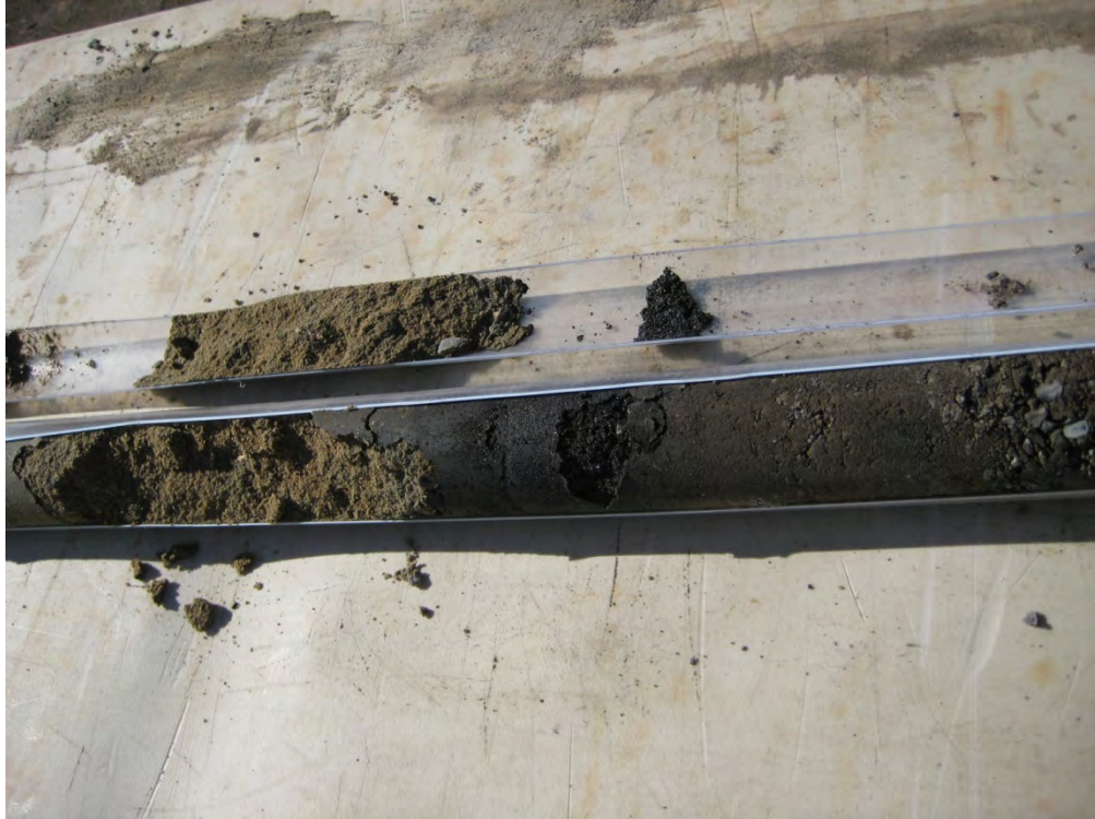
Photograph 4. Soil boring location FS-09d showing sandblast grit at 1 foot bgs.
