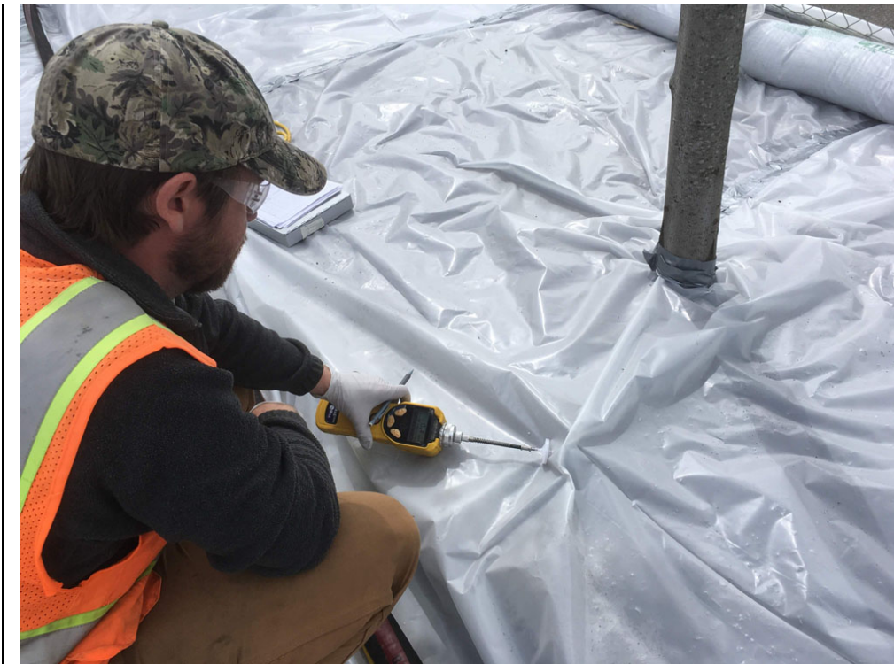
Photo #13: Measuring airspace beneath the visqueen near AS-1 with a PID. Readings beneath the visqueen were similar to ambient.
