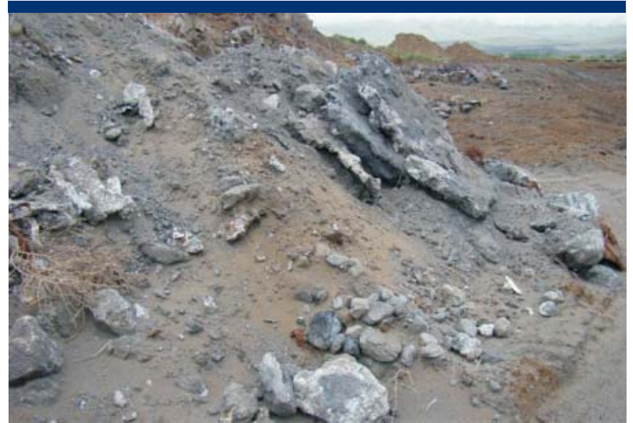
Photo 6 Aluminum waste inclusions, clast sizes several feet across. Direction: Northeast Date: 5/6/09
