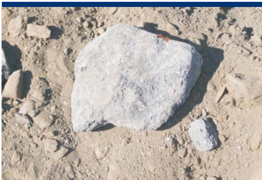
Photo 19 Spent potliner black, carbon, relatively light. K088 waste stream. Typical example, covered with gray dust.
