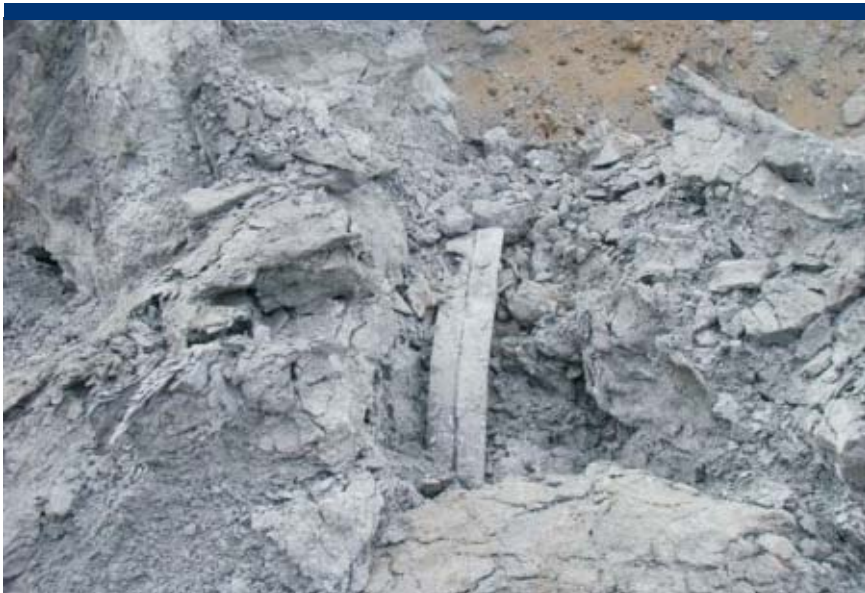
Photo 7 Dross material left exposed to dessicate for easier crushing. Direction: Down Date: 5/6/09
