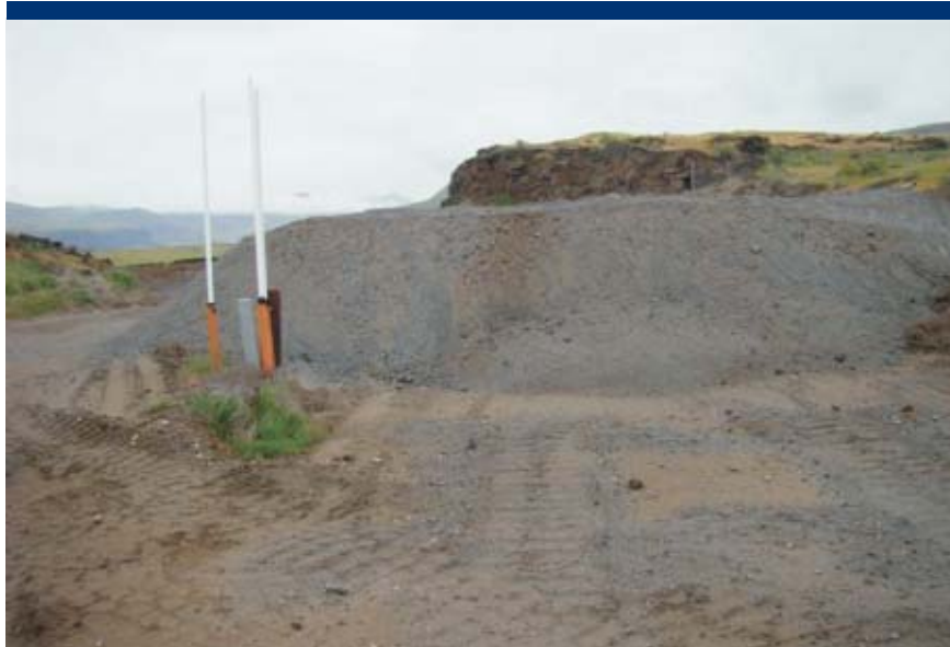
Photo 1 Monitoring well MW-1 (abandoned) at the west end of landfill. Stockpile of crushed dross behind well.
