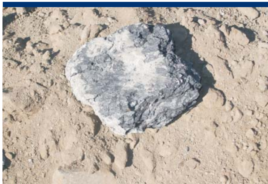
Photo 20 Spent potliner black, carbon, relatively light. K088 waste stream. Example with visible black carbon.
