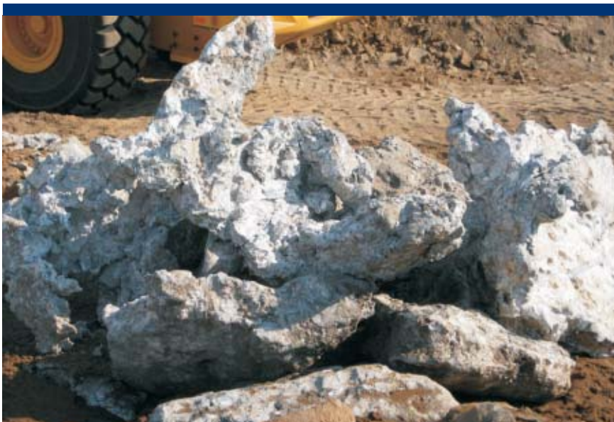
Photo 15 Aluminum dross (white dross, metallic form), a by-product of primary aluminum smelting. Chunks of aluminum/metal, silver/gray, dense, high metal content.
