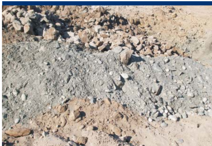
Photo 16 Aluminum dross (white dross, powder form) Silver/gray, powdery. Non-hazardous waste stream.
