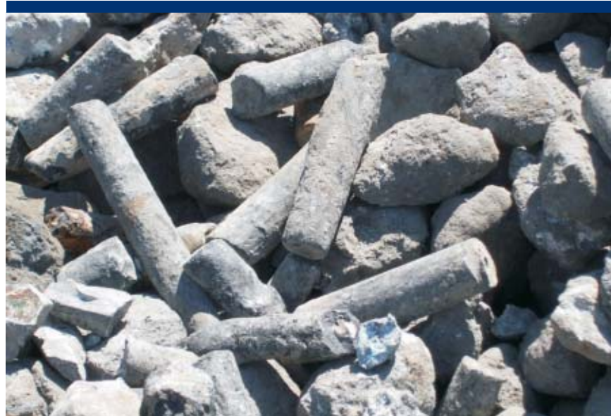
Photo 18 Anodes (cylinders/rods) and spent potliner. Black, carbon, relatively light. K088 waste stream.
