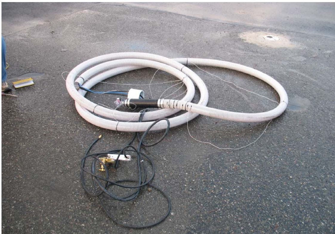
Photograph 1. The Plume Eater™ Technology system well insert, prior to down-well placement.
