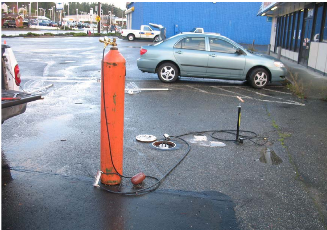
Photograph 2. The Plume Eater™ Technology system injecting helium during pilot test.
