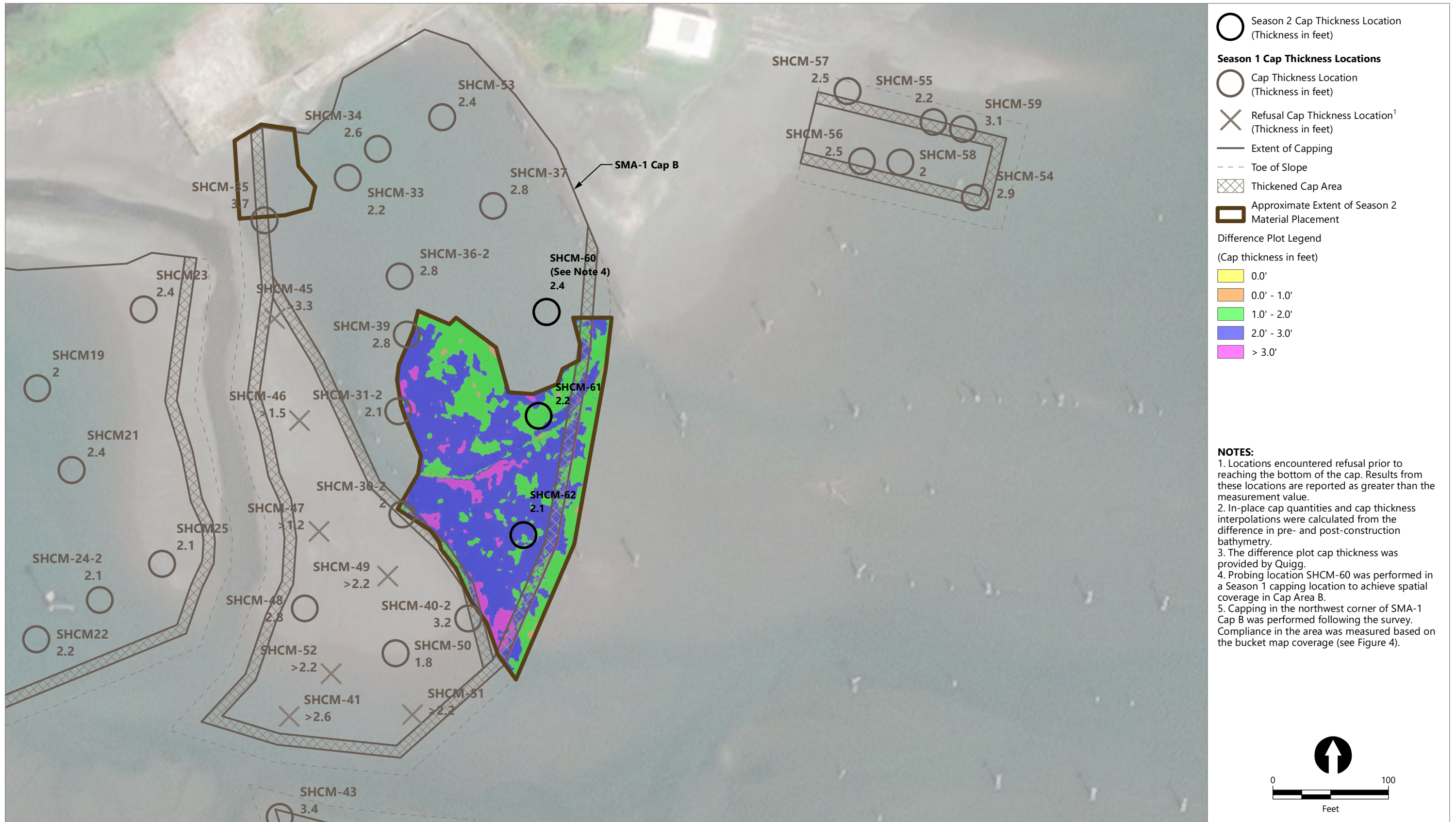
Figure 2 Cap Thickness and Probing Locations – SMA-1 Cap B Shelton Harbor Interim Action: Season 2 Water Quality and Cap Thickness Monitoring Oakland Bay and Shelton Harbor Sediments Cleanup Site
