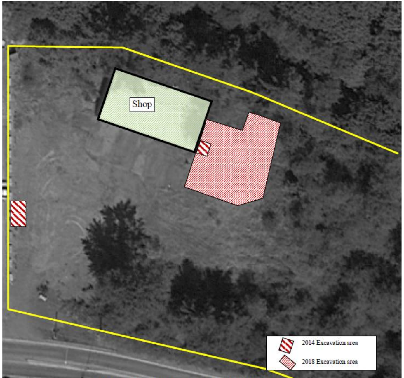
Figure 9. Horizontal Extent of soil contamination
