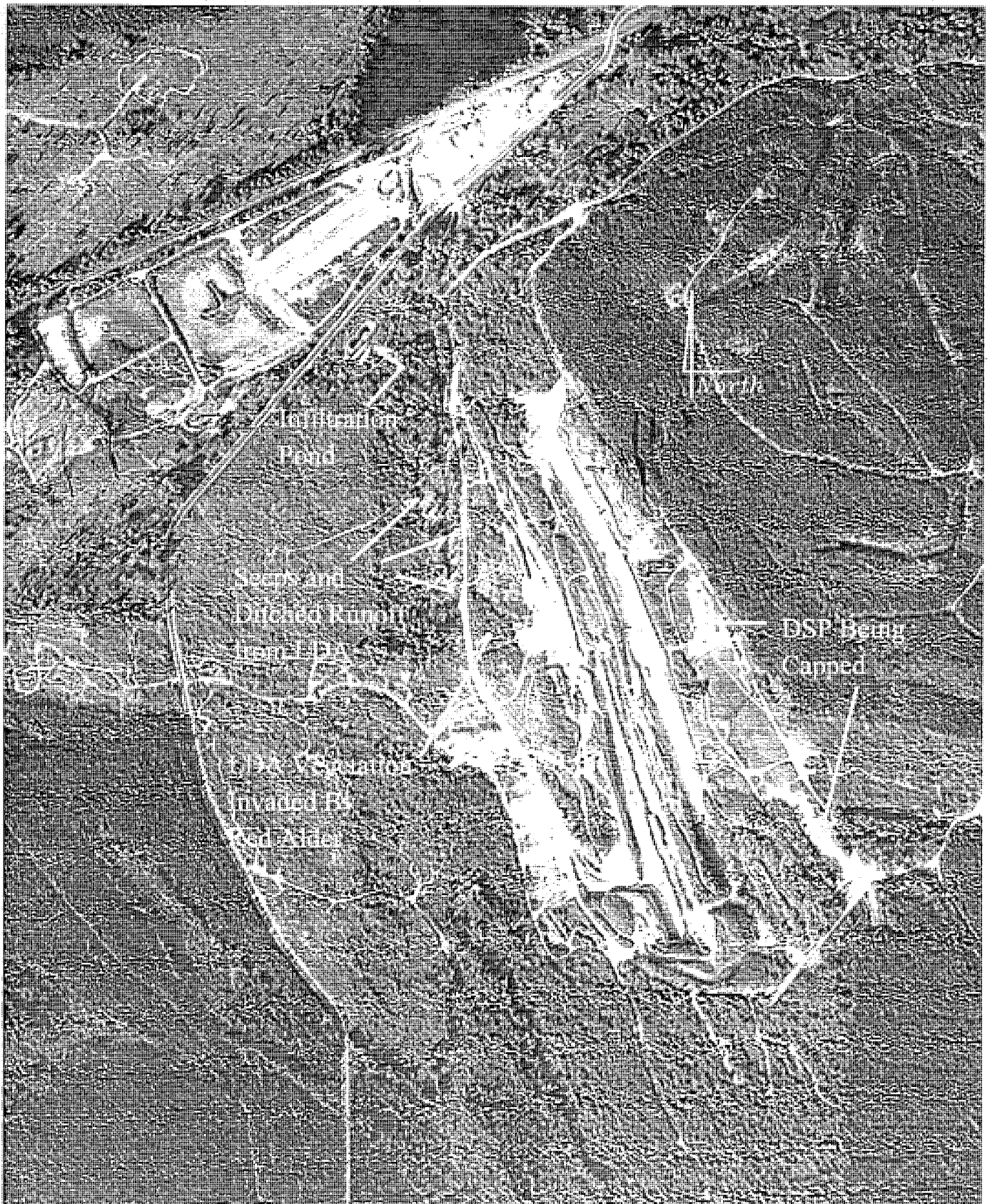
Photo 1-4. 1995 aerial photograph of Ravensdale site. Showing completed landfilling of Dale Strip Pit (DSP). Grading of DSP cap is in progress. Seeps and pooled leachate are present at Lower Disposal Area (LDA). Infiltration ponds can be seen northwest of LDA. Woody vegetation has invaded LDA cap.
