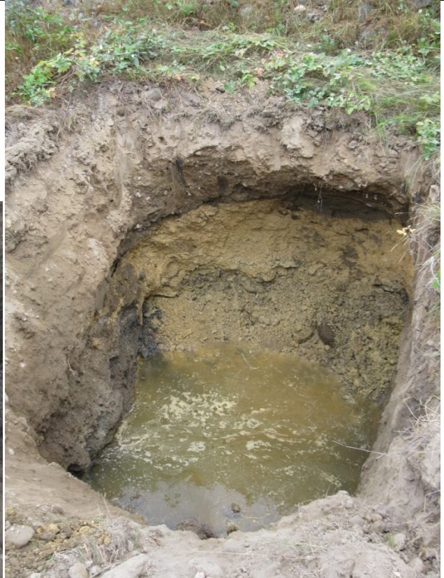
Gravel lens and water in Test Pit #2 tested today.
