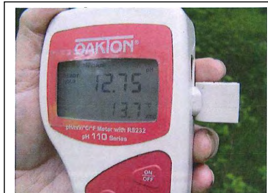
WA Department of Ecology monitoring photo: "Description: pH meter reading of hard-pipe discharge [i.e., leachate discharging from collection system]. (WDOE Water Quality Program. Recommendation for Enforcement Action. June 21, 2016.)
