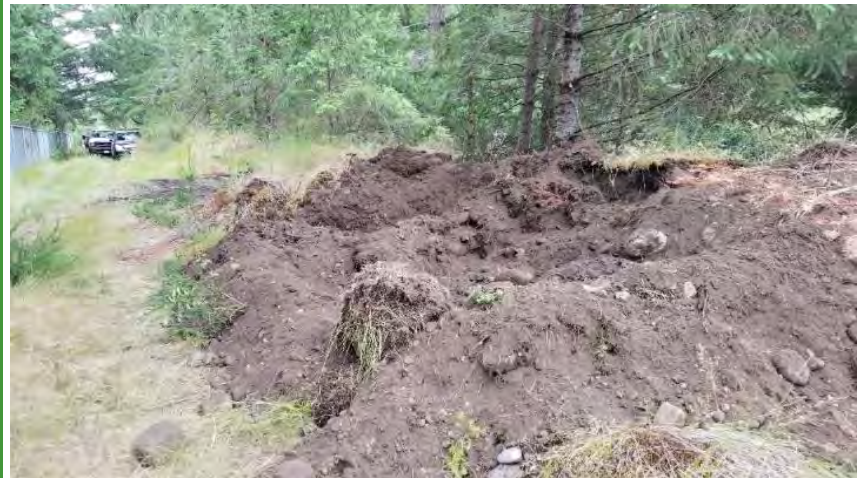
22. Test Pit G with petroleum stained soils.
