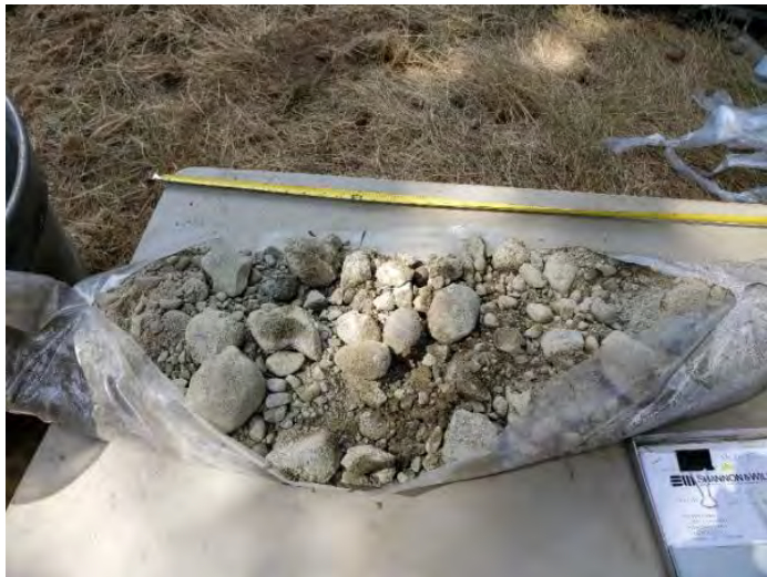
32. MW-1 representative soils (e.g., gravel with sand at 10 to 15 feet below ground surface (bgs)).
