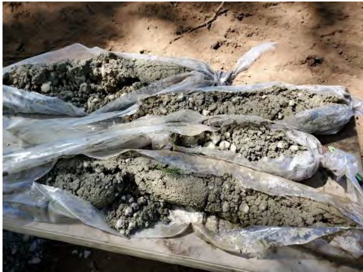
36. MW-3 saturated soils from 40 to 50 feet bgs.
