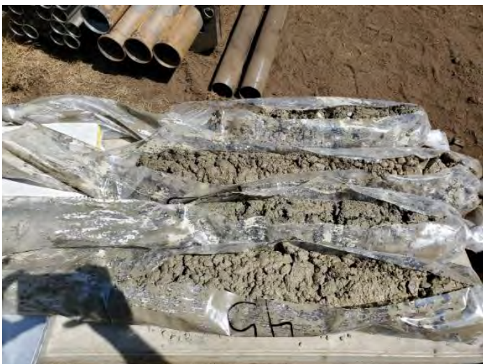
34. MW-2 saturated soils from 40 to 45 feet bgs.
