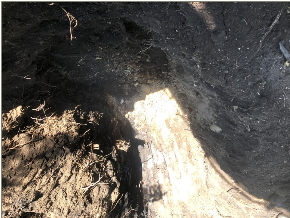
Photograph 10: TP-9 was excavated to 8 feet below ground surface. This is when outwash was observed.
