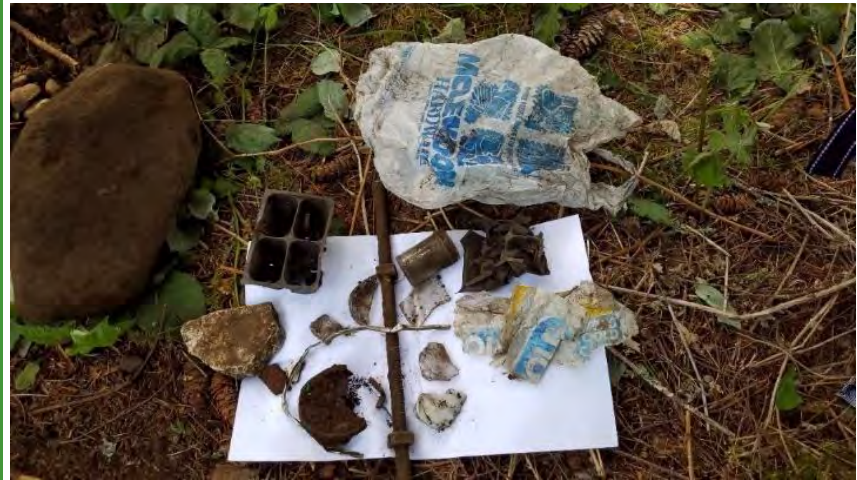
10. Test Pit A debris (black plastic seedling trays, glass, porcelain, brick, tin can, metal screen edging, plastic bags, steel threaded rod, and concrete).
