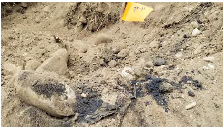
23. Test Pit H with petroleum stained soils and clothing.
