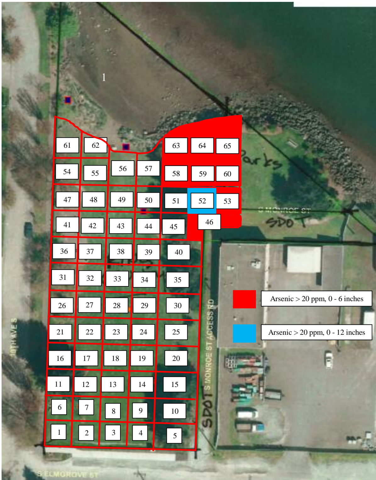
Figure 1. Soil sampling grids with arsenic above the Ecology cleanup standard of 20 ppm. Duwamish Waterway Park, Seattle. January, 2019.
