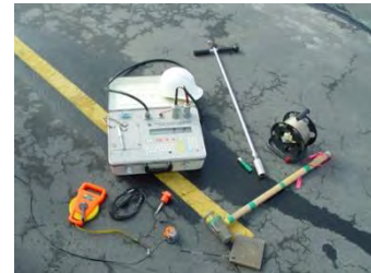
Figure 1 seismograph and field equipment
