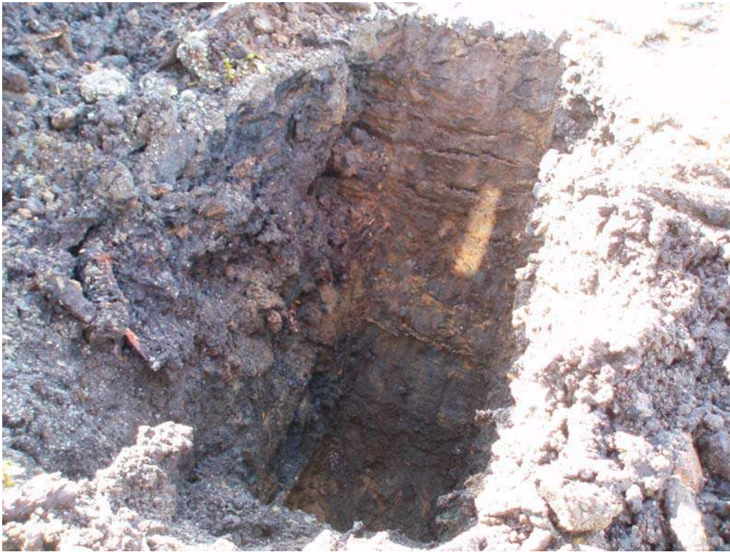
Photograph 9 – View into 8-foot-deep excavation at Test Pit 2
