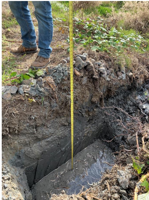
Photograph 4. TP-3 at total depth of 6 feet.
